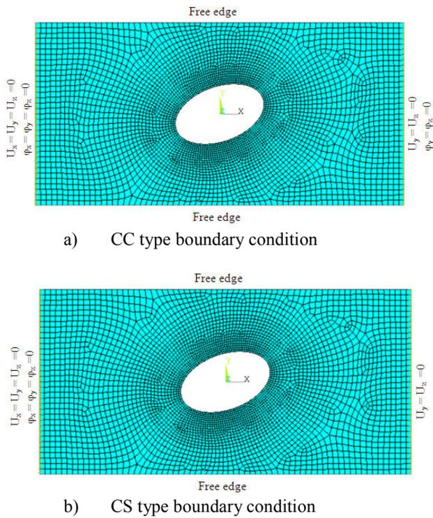
Fig.3 .Boundary conditions and finite element mesh of the laminated plate
