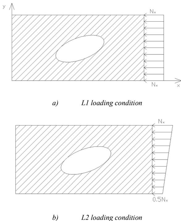
Fig.4. Details various loading conditions
