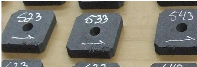
Fig. 10 Example of uncut fibers produced from the cross cut cutting tools
