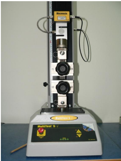
Figure 14 – Universal testing device (Multitest 5-I, Mecmesin Ltd, UK)
