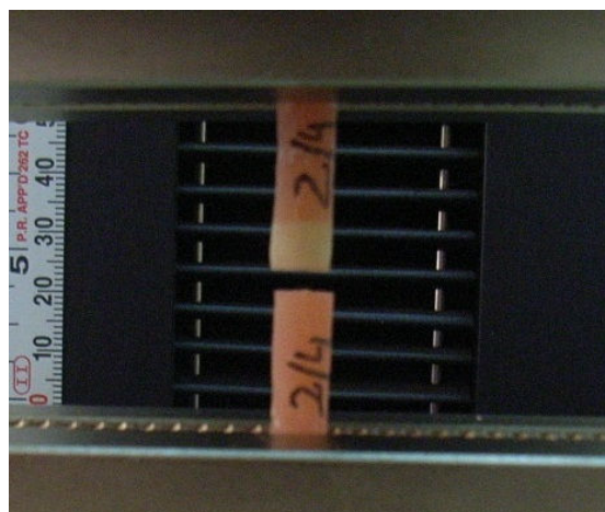
Fig. 16. Sample fixed to the Mecmesin holding device before after the adhesive fracture
