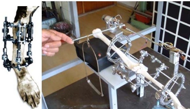
Fig. 3 Application of external fixator (treatment of a dog, treatment of a human - experiments in the laboratory at VSB – Technical university of Ostrava)
