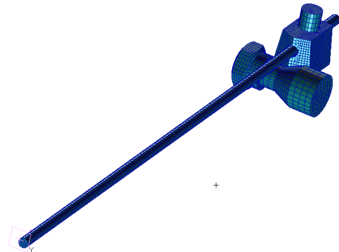
Fig. 18 Numerical modelling (FEM - Kirschner wire and detail of its attachment).
