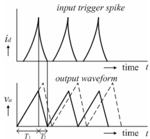
Fig. 7 Astable pulse generator with external injection. Dotted line is an original waveform. Solid line is a synchronized waveform to input trigger pulse.
