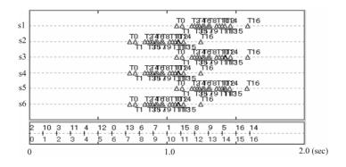
Fig. 6 Estimated and actual generation times. Upper: sequences of arrival pulse times at each sensor. Below : Actual(upper) and estimated(lower) time of pulse generations.
