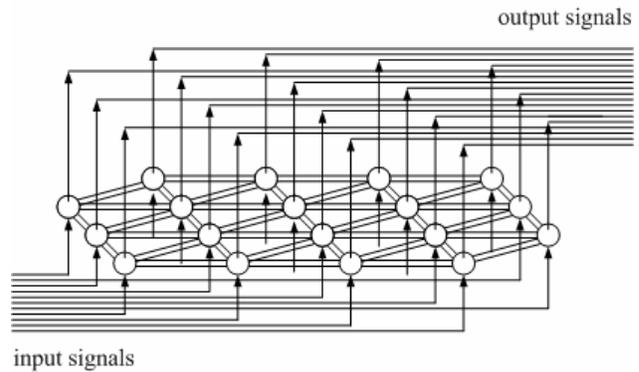
Fig. 3 Formulation of a neural system with mutual connections. Circle shows a neuron. Double solid lines denote mutual connections.
