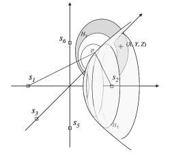
Fig. 1 Principle of the Hyperboloid Method in 3D space. The third hyperboloid is abbreviated.
