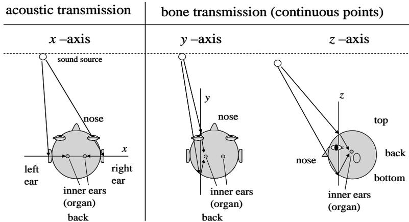
Fig. 2 Reception of sound signals in 3D space by phase delay defined along x, y, z axes.
