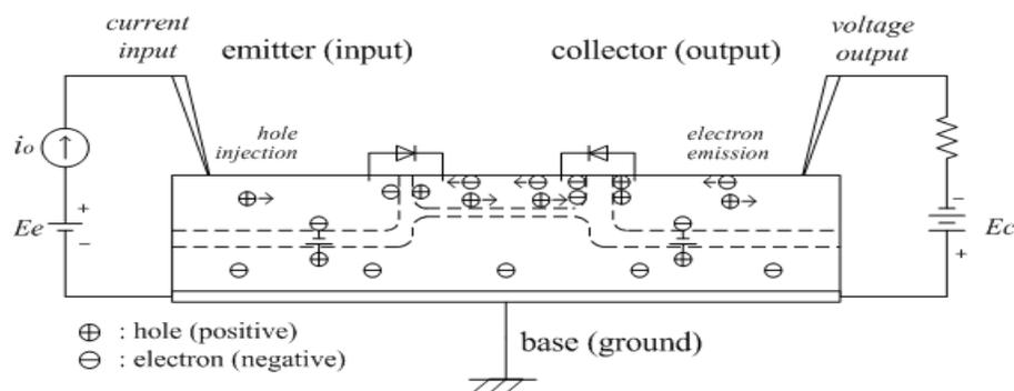
Fig. 9 Electro-physical modeling of Point Contact Transistor (PCT).
