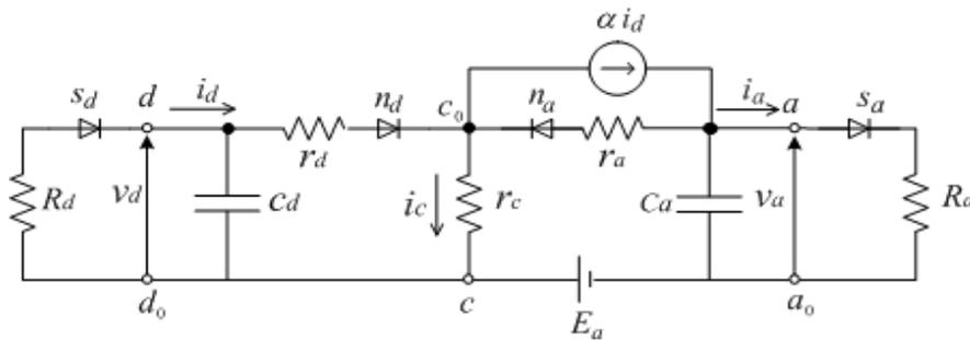
Fig. 5 Electrical modeling of an active neuron.
