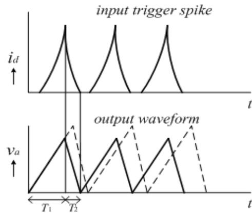
Fig. 6 Astable pulse generator by external injection. Dotted line is an original waveform. Solid line is the waveform synchronized to input trigger pulse.
