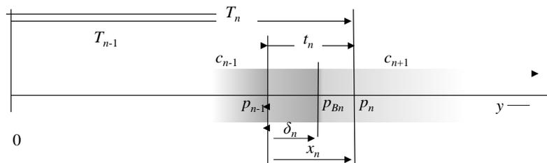
Fig.4 Structure of a section  $n$  with a boundary at point  $p_{Bn}$ .
