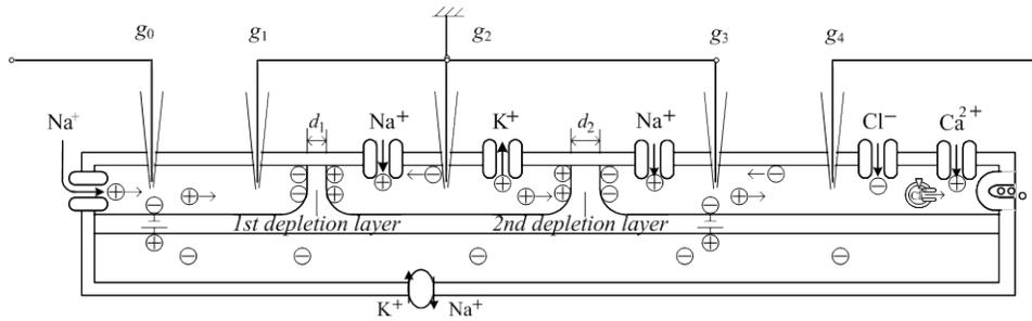
Fig. 1 Electro-physical modelling of an active neuron for positive pulse generation.  $g_0 \sim g_5$  are small glass electrodes to be inserted in a neuron for electrical measurement. A pair electrodes in each zone are first inserted.
