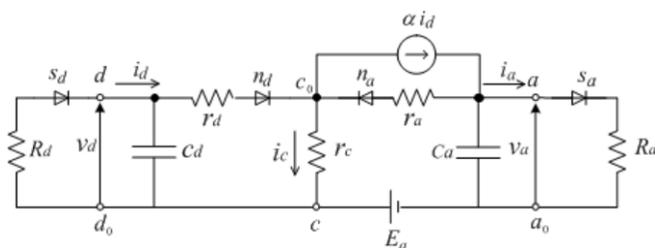
Fig. 3 Electrical modeling of an active neuron for positive pulse generation.
