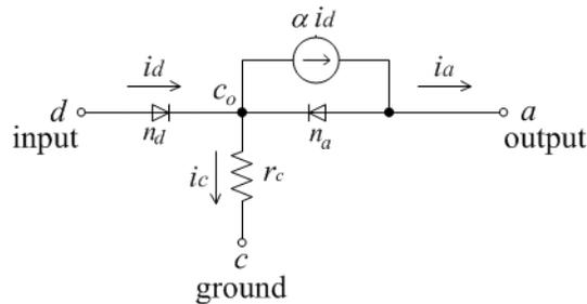
Fig. 2 Electrical modeling of activity of a neuron for positive pulse generation.
