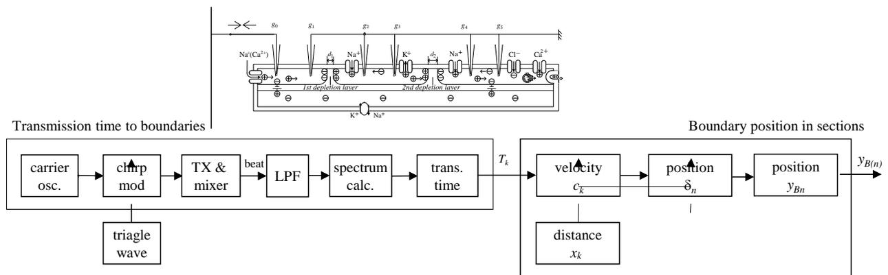
Fig. 5 System configuration of electrical measurement scheme. Transmission times to boundaries measured by the chirp method. Positions of boundaries are measured by the proposed method.
