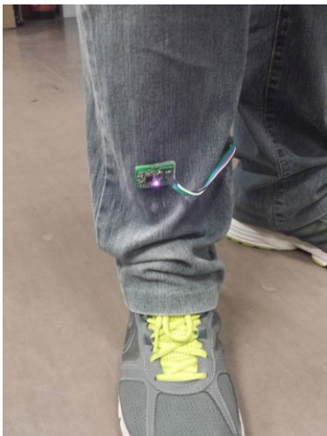
Fig. 2 - Installation positions of the IMU
