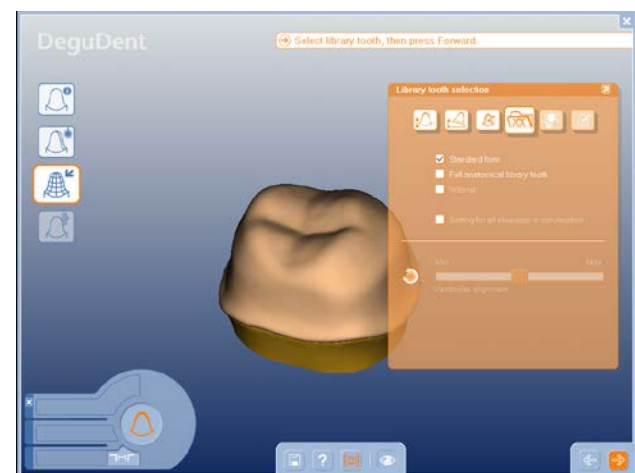
Fig. 2. Design of a standard form framework (uniform thickness of 0.5 mm)
