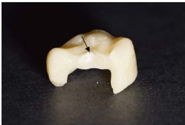
Fig. 4. Fracture surface of a pressed ceramic crown specimen exposing fracture origin on the occlusal loading point and the fractographic map.
