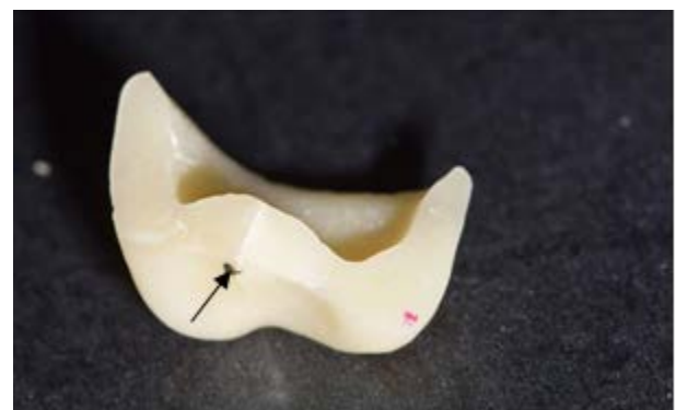
Fig. 7. Fracture surface of a pressed ceramic crown specimen exposing fracture origin on the occlusal loading point and the fractographic map.
