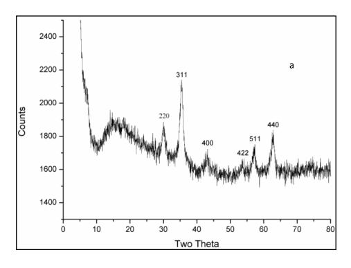
Fig 3: XRD of (a) iron oxide nanoparticle and (b) pectin coated iron oxide nanoparticle.
