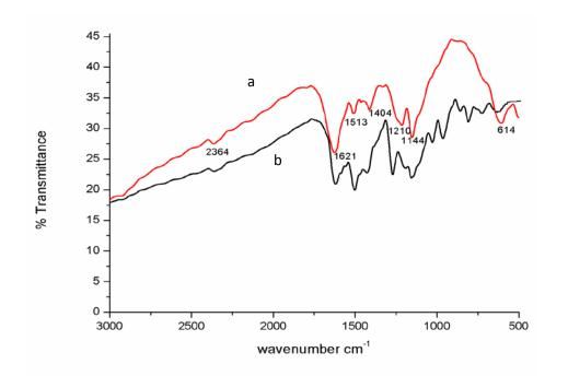
Fig 2 FTIR spectra of (a) curcumin and (b) curcumin conjugated pectin coated iron oxide nanoparticles.
