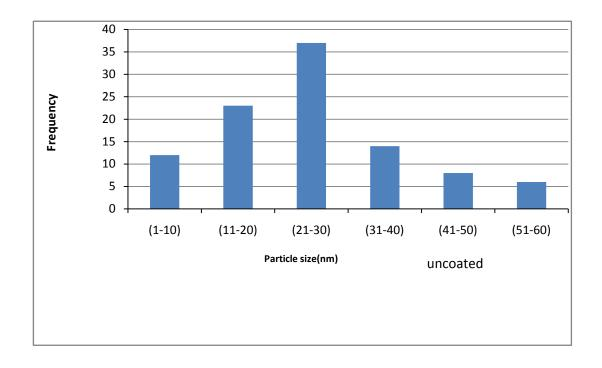
Fig.6 The particle size distribution for both uncoated and coated iron oxide nanoparticles.
