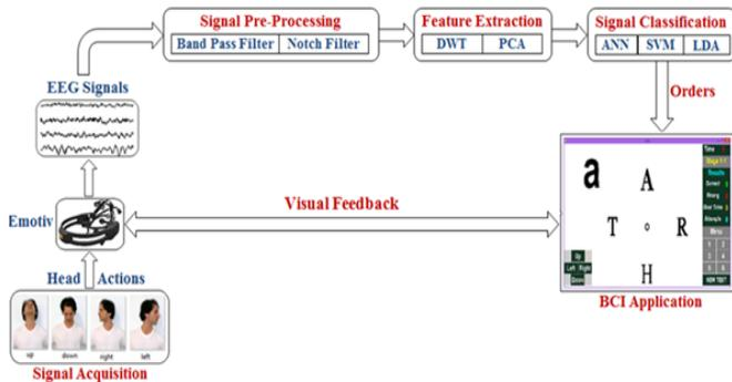
Fig. 10 the block diagram of the BCI system
