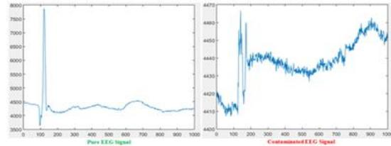
Fig. 4 pure EEG signal and contaminated EEG signal for head movement to the left
