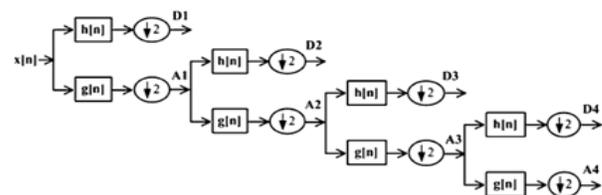
Fig. 5 sub-band decomposition of DWT:  $h[n]$  is the high-pass filter and  $g[n]$  the low-pass filter [39]
