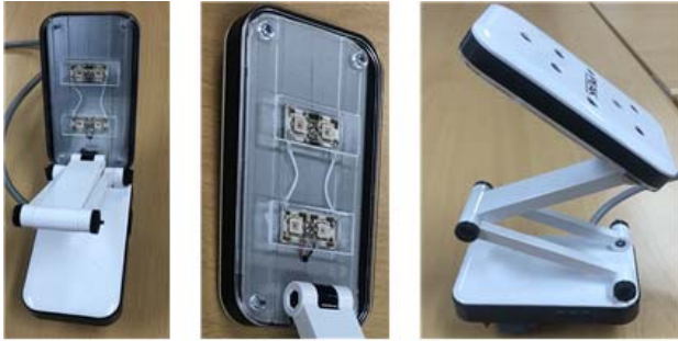
Fig. 5 Developed UVB-LED special lighting
