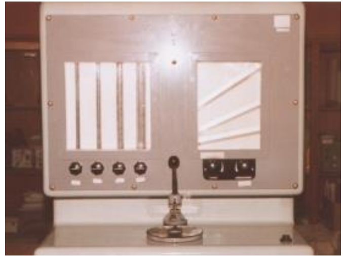
Figure 11: Facility Metefem FF-12/A for measuring the permeability of fabrics [20]
