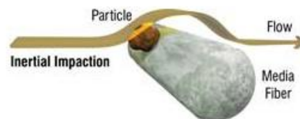
Figure 7: Representation of the principle of capturing particles in the fiber – The inertial impaction [3]
