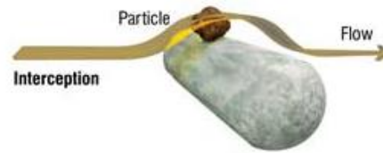
Figure 6: Representation of the principle of capturing particles in the fiber – The interception [3]
