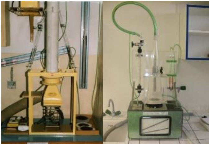
Figure 10: Facility no. 1 for testing by means of synthetic dust Name: DFT-2 (Dust Filter Tester), DFT-3 [20]
