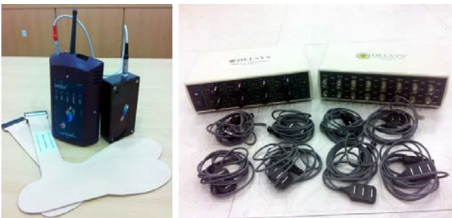
Fig. 6. Pedar X-system and Delsys EMG system
