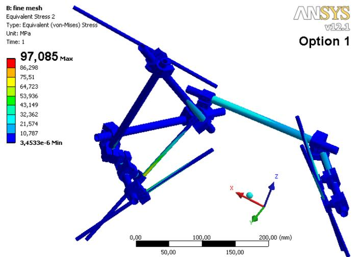
Fig. 12 “Option 1” - FE modelling of external fixator for pelvis and acetabulum (equivalent von Mises stresses /MPa/ for tensile loading 100 N)
