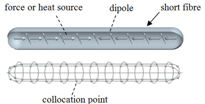
Fig. 1 Distribution of source functions and collocation points
