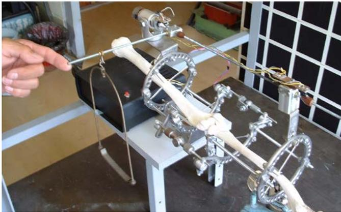
Fig. 15 Experimental measurements - external fixator (Ilizarov apparatus)
