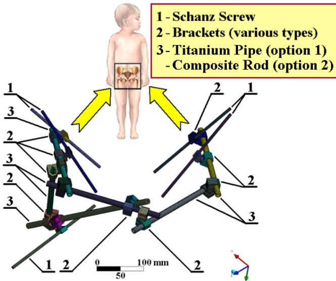
Fig. 10 Application of external fixator for treatment of pelvis and its acetabulum
