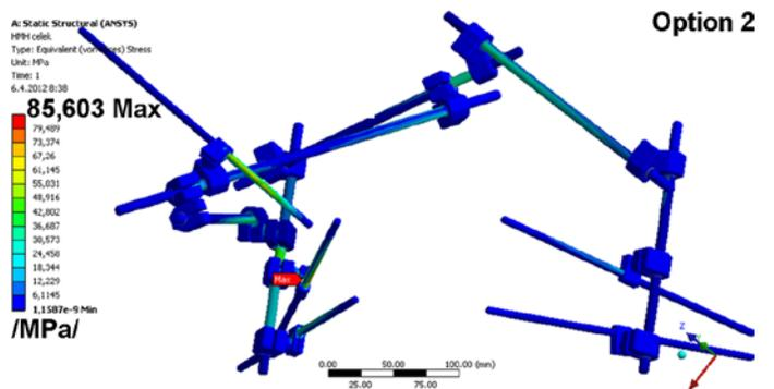
Fig. 13 “Option 2” - FE modelling of external fixator for pelvis and acetabulum (equivalent von Mises stresses /MPa/ for tensile loading 100 N)
