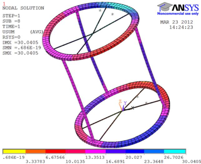
Fig. 14 FE modelling of external fixator - Ilizarov apparatus (overloading, total displacements in the structure)
