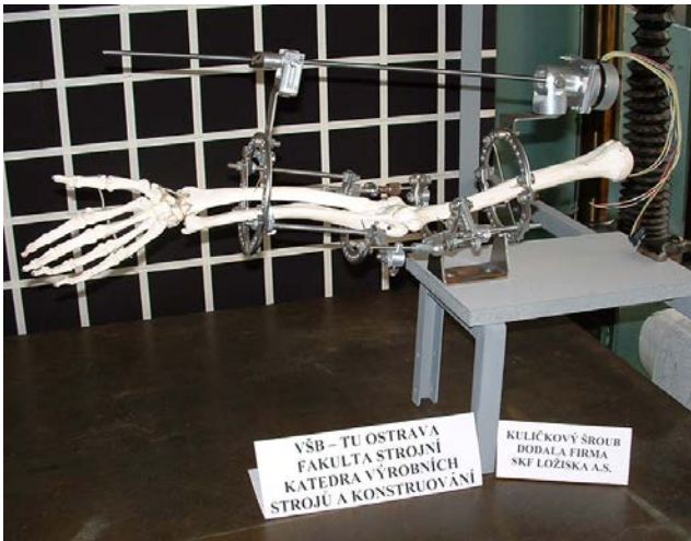
Fig. 6 Prototype of the designed external fixator with the stepper motor and movement screw with the ball nut
