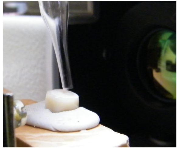
Fig.No.6. One of the acrylic samples in front of the OCT device scanning head during acetone treatment.
