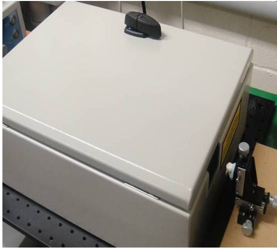
Fig.No.5. Time Domain OCT device used to investigate the effect of acetone to acrylic teeth.
