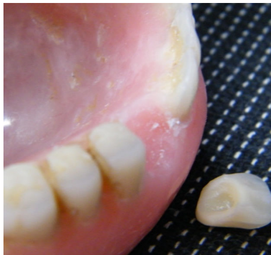
Fig.No.1. Dethachment of acrylic teeth from denture base resin
