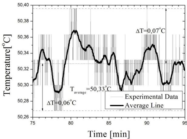
Fig.23 – Internal temperature oscillation when an external disturbance is forced.
