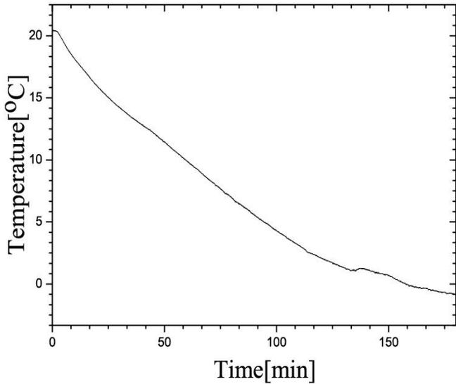
Fig.15 – Variation of temperature with time when the thermal chamber is set to 0°C.
