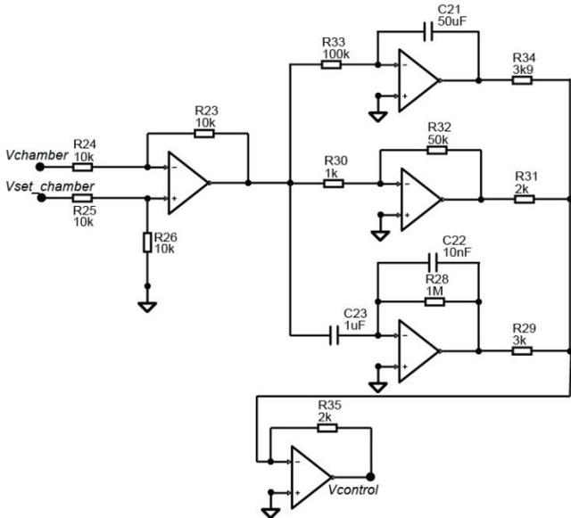
Fig.6 – PID circuit used for the bottom TEM control.
