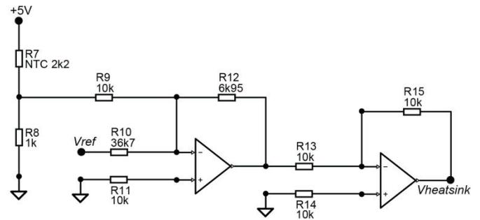
Fig.4 – NTC signal conditioning circuit.
