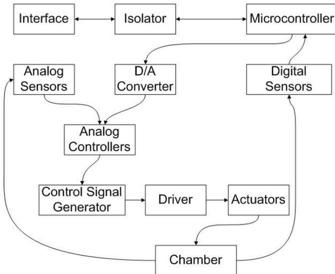
Fig.3 – Block diagram of the thermal chamber circuits.
