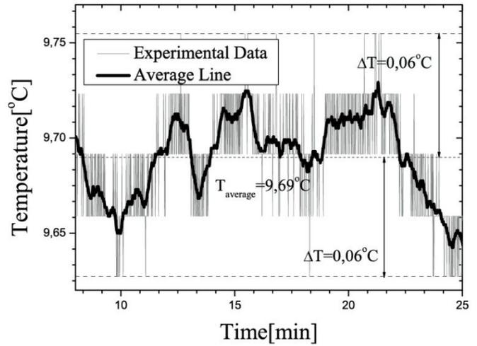
Fig.21 – Internal temperature oscillation when an external disturbance is forced.
