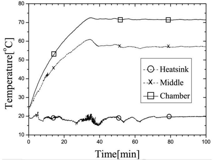
Fig.17 – System temperature graph for 70°C set.
