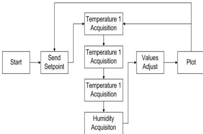
Fig.10 – Block diagram of the user interface software.
