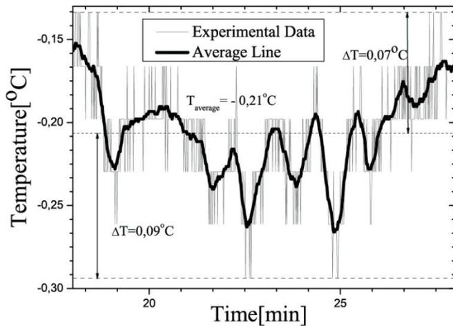
Fig.16 – Temperature variation near 0°C.
