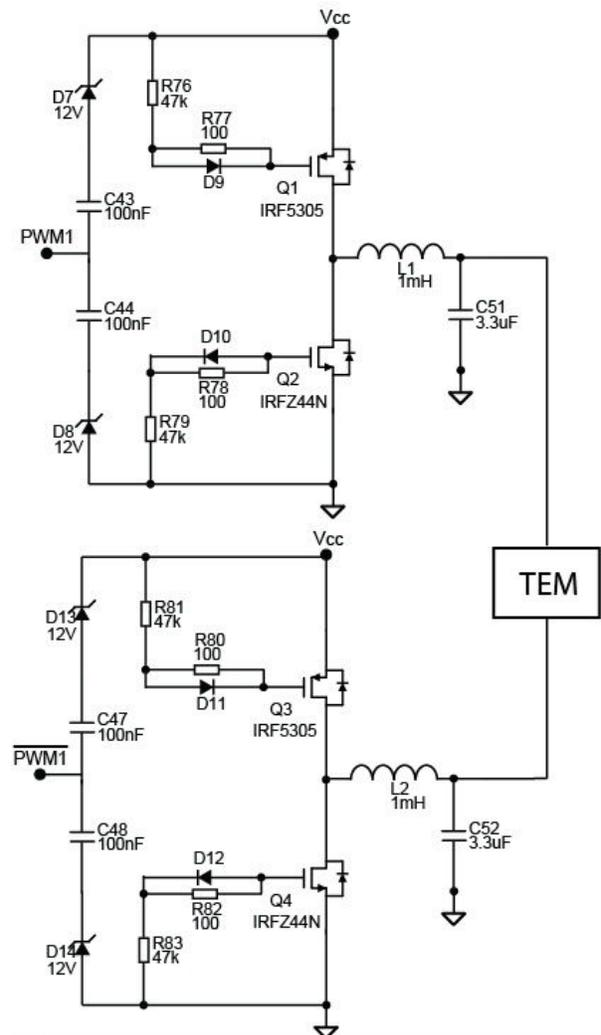
Fig.9 – PID circuit used for the bottom TEM control.
