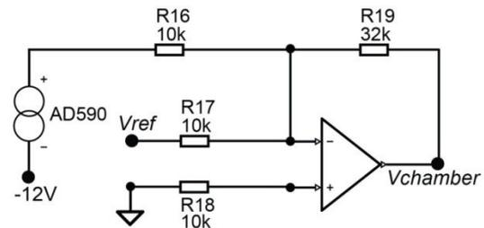
Fig.5 – Conditioning circuit for the AD590.
