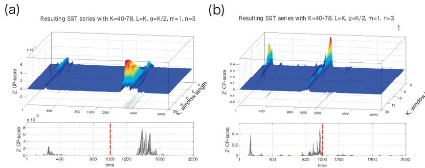
Fig. 8. (a) The resulting conventional SST series for the test data 1 shown in the right panel of Fig. 6. (b) The resulting multivariable SST series for the test data 1 shown in the right panel of Fig. 6. SST parameters were set to  $K = 40-78$ ,  $L = K$ ,  $g = K/2$ ,  $m = 1$  and  $n = 3$ . The vertical dashed line shown in red indicates the onset time of the precursory event.
