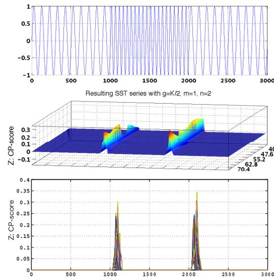
Fig. 5. Upper panel: Original data generated using sine functions whose frequency changes at  $t = 1000$  and  $t = 2000$ . Lower panel: The resulting conventional SST series with  $K = 40-78$ ,  $L = K$ ,  $g = K/2$ ,  $m = 1$  and  $n = 3$ .
