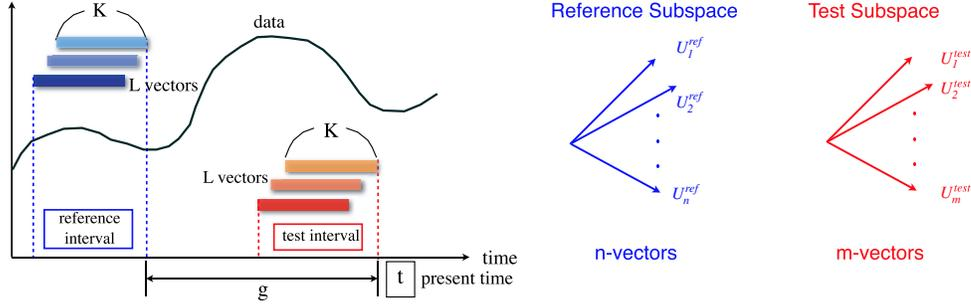
Fig. 4. (Left panel) A diagram of pattern extraction by conventional SST. From  $L$  subsequences at both side of present time  $t$ , *representative patterns* are calculated. (Right panel) A diagram of the reference subspace and the test subspace. Change-point score is defined by using the angle between these two subspaces.
