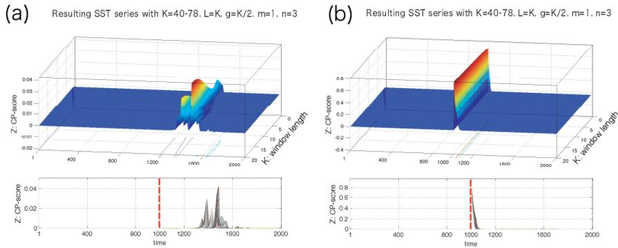
Fig. 7. (a) The resulting conventional SST series for the test data 1 shown in the left panel of Fig. 6. (b) The resulting multivariable SST series for the test data 1 shown in the left panel of Fig. 6. SST parameters were set to  $K = 40-78$ ,  $L = K$ ,  $g = K/2$ ,  $m = 1$  and  $n = 3$ . The vertical dashed line shown in red indicates the onset time of the precursory event.
