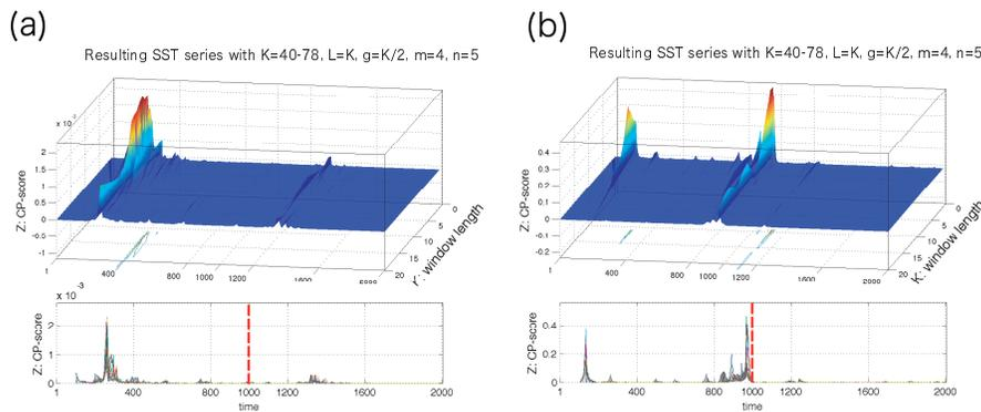
Fig. 9. (a) The resulting conventional SST series for the test data 1 shown in the right panel of Fig. 6. (b) The resulting multivariable SST series for the test data 1 shown in the right panel of Fig. 6. SST parameters were set to  $K = 40-78$ ,  $L = K$ ,  $g = K/2$ ,  $m = 4$  and  $n = 5$ . The vertical dashed line shown in red indicates the onset time of the precursory event.
