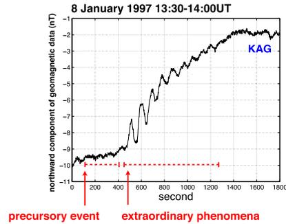
Fig. 1. Northward component of geomagnetic data around an auroral substorm onset observed at KAG station.
