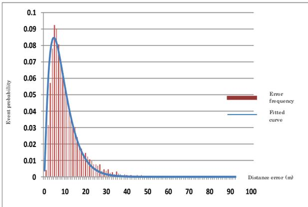
Fig. 16 The frequency of errors and the approximate Gamma curve (Outdoor example)
