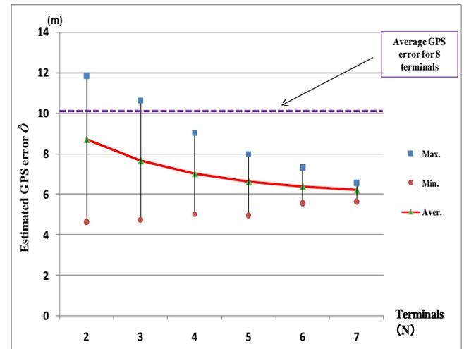
Fig. 19 The relationship between the number of terminals,  $N$ , and the estimated error in the case for temporary value position
