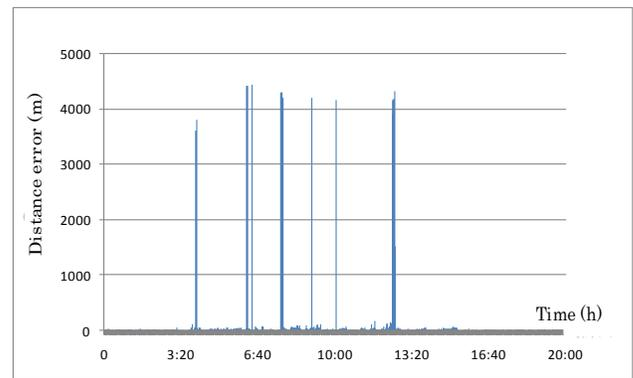
Fig. 9 Indoor impulse noise measurement results with terminal 4-C-2 (same terminal type as 4-C-1)
