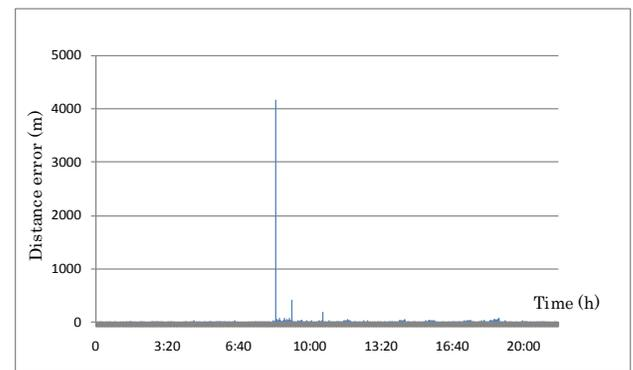
Fig. 11 Indoor impulse noise measurement results with terminal 3-C
