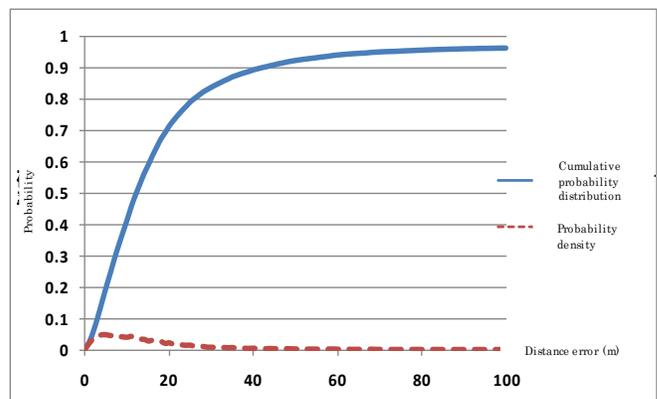
Fig. 16 Cumulative probability distribution of GPS errors (Indoor)
