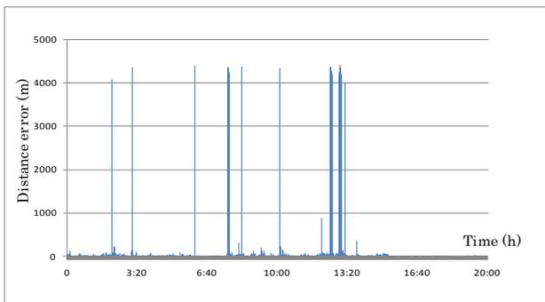
Fig. 8 Indoor impulse noise measurement results with terminal 4-C-1 (same terminal type as 4-C-2)
