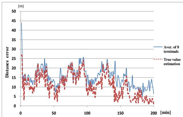
Fig. 18 Comparison of the average distance error of the true value estimation method using 8 mobile phone terminals
