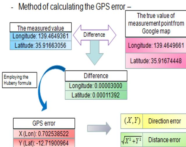
Fig. 3 Process of calculating the GPS error
