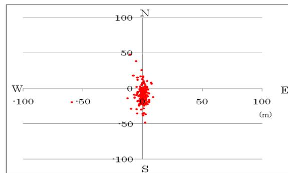
Fig. 4 Error variance diagram for the Eastern direction
