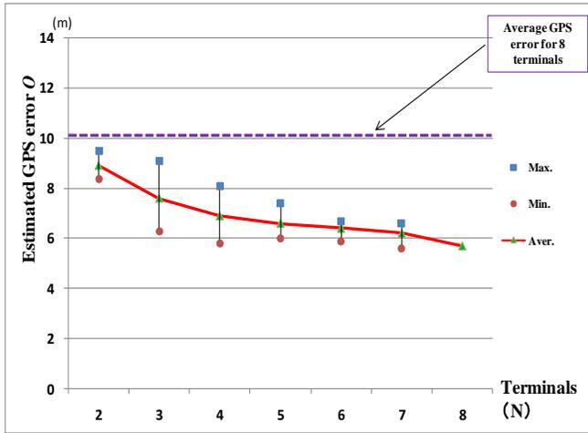
Fig. 17 The relationship between the number of terminals,  $N$ , and the estimated error in the case for true value position
