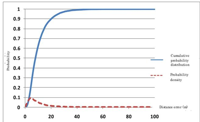
Fig. 15 Cumulative probability distribution of GPS errors (Outdoor)
