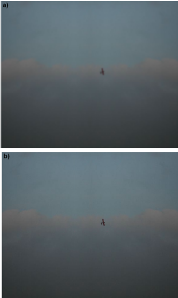
Fig. 3 The results of unblait operation applied to the image obtained by vision system: a) image recorded by the thermo-optical set, b) image after unblait operation
