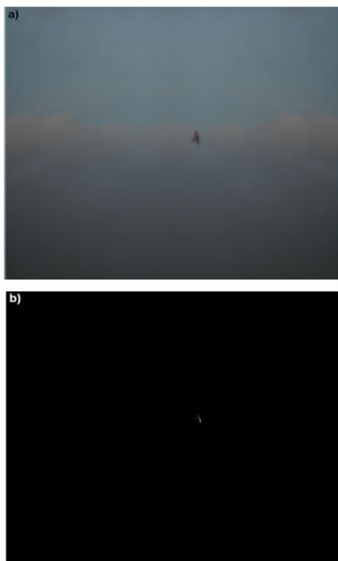
Fig. 4 Results of using Sobel's filter: a) image acquired from visual system, b) image after filtering using Sobel's filter
