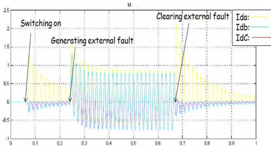
Fig.6 Differential currents during switching on the transformer and an external fault.
