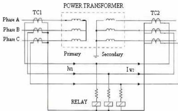
Fig.1 Typical differential power transformer protection relay
