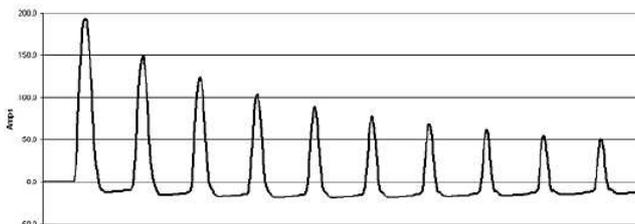
Fig 2: Transformer Inrush (One Phase).
