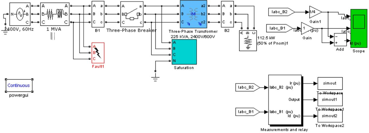
Fig. 5 The system Simulink model.
