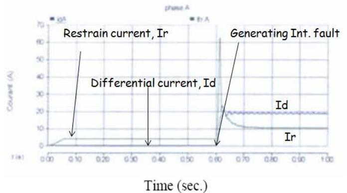
Fig. 7 Differential and restrain current signals.
