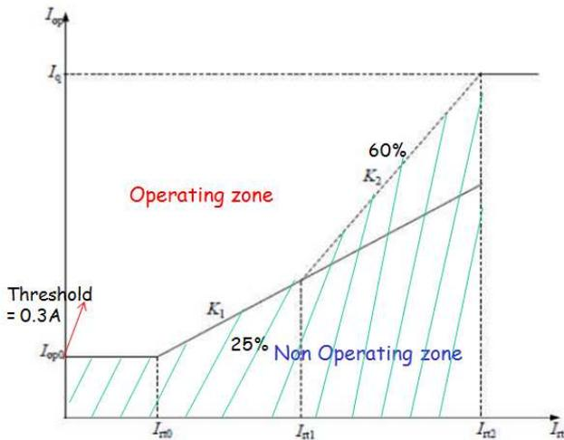
Fig.4 Characteristics of differential relay.
