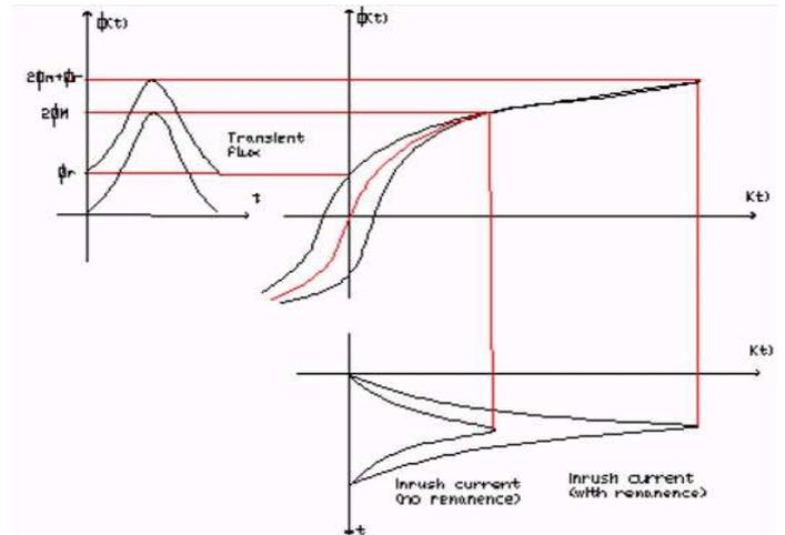
Fig.3 Typical curve of fluxes and inrush current.
