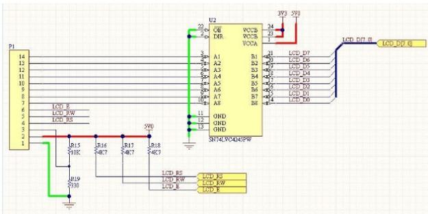
Fig. 13 Liquid Crystal Display schematic diagram
