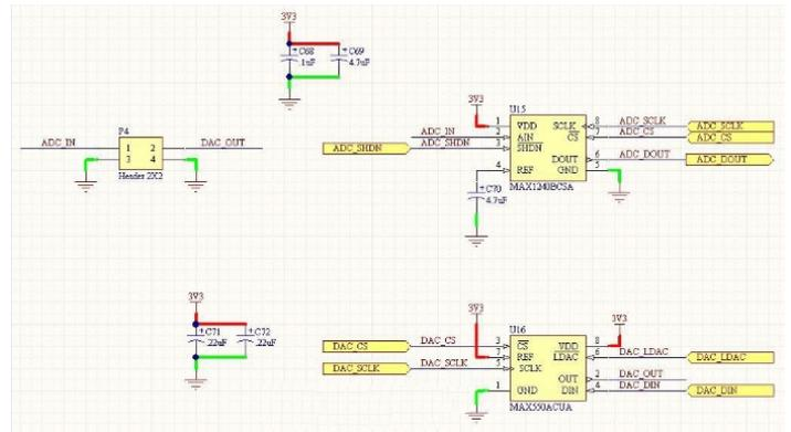
Fig. 11 ADC/DAC schematic diagram
