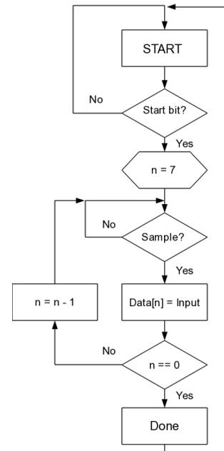
Fig. 6 UART Receive Process
