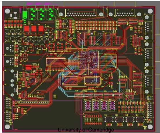
Fig. 1 Motherboard PCD Layout Diagram
