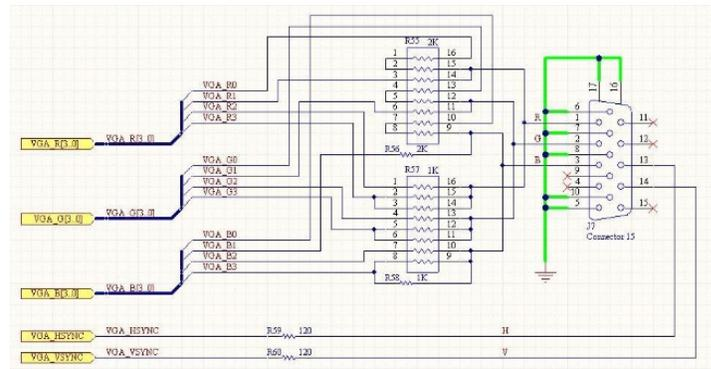
Fig. 3 VGA Port Schematic Diagram
