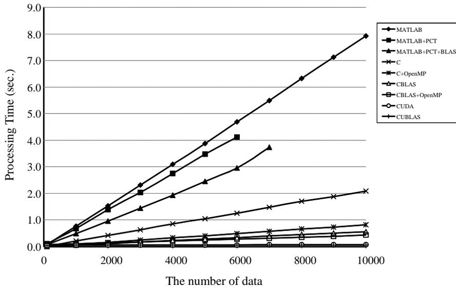
Fig. 5. Computational costs versus the number of data (pixels) to be classified. Experimental conditions:  $k=9$  ( $3 \times 3$ ), and  $k'=9$ .
