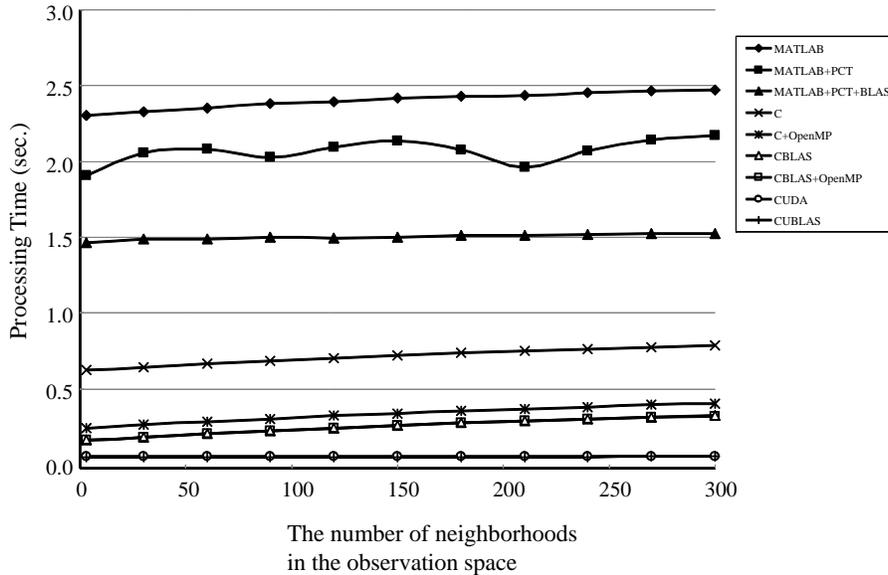
Fig. 6. Computational costs versus the number of neighboring data (pixels) in the data observation space to be classified. Experimental conditions: the number of data to be classified is 3,000, and  $k'=9$ .
