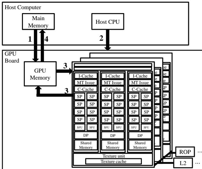
Fig. 4. Architecture of GPU computing board and execution process of GPGPU.
