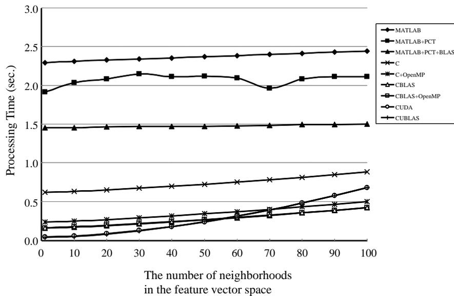
Fig. 7. Computational costs versus the number of neighboring vectors in the feature vector space. Experimental conditions: the number of data to be classified is 3,000, and  $k=9(3 \times 3)$ .
