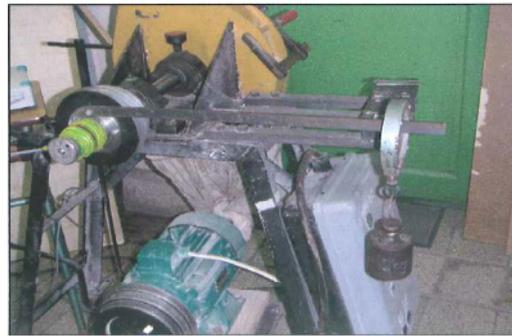
Fig. 9 torque transducer calibration using deadweights
