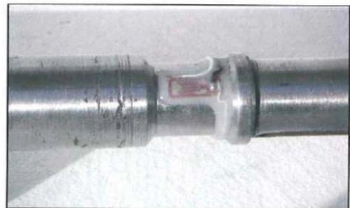
Fig. 6 V-shaped strain gauge mounted on a shaft
