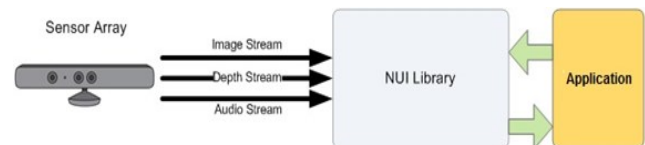
Fig. 6 Hardware and software interaction with an application [10]
