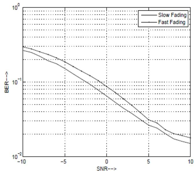
Figure 10: BER curve showing flat fading versus slow fading for BPSK..
