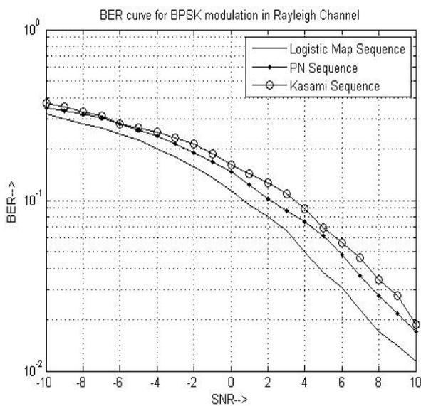
Figure 7: BER curve for BPSK Modulation in Rayleigh Channel.
