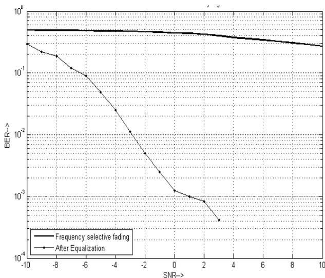
Figure 23: BER curve showing frequency selective fading.
