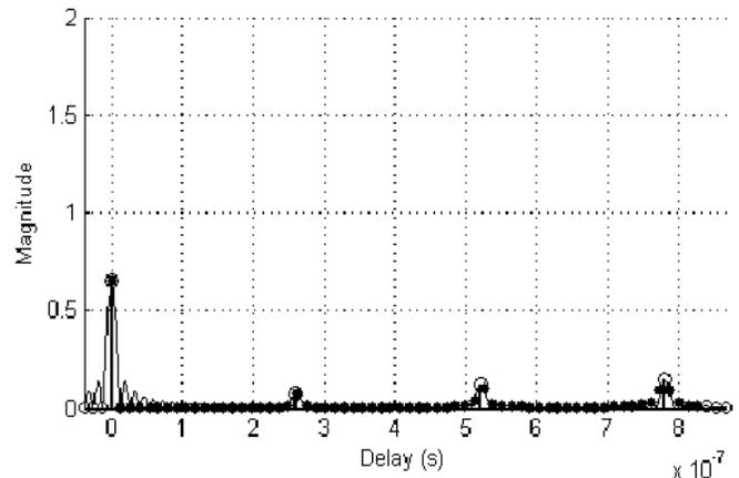
Figure 24: Channel Impulse response for frequency selective fading channel.
