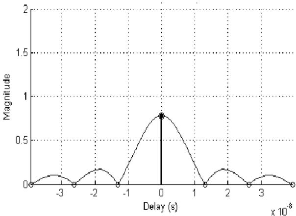
Figure 22: Channel Impulse response for fast fading channel.
