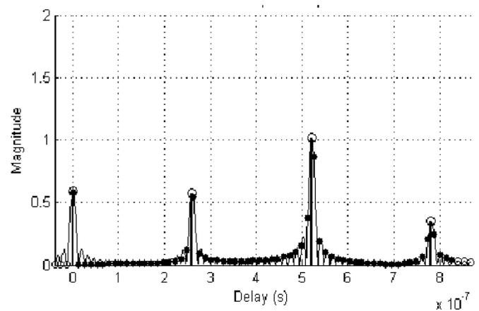
Figure 14: Channel Impulse response for frequency selective fading channel.
