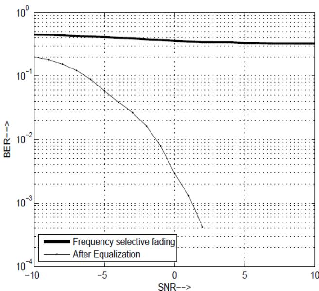
Figure 13: BER curve showing frequency selective fading.
