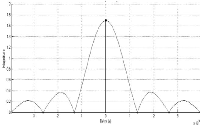
Figure 11: Channel Impulse response for slow fading channel.
