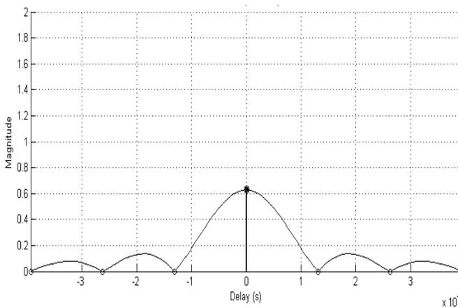
Figure 12: Channel Impulse response for fast fading channel.
