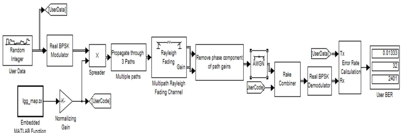
Figure 28: System model for Rayleigh Channel.
