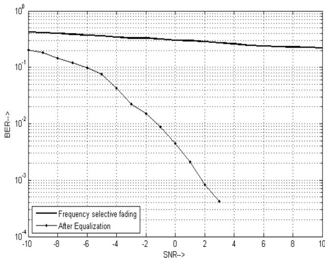
Figure 18: BER curve showing frequency selective fading.
