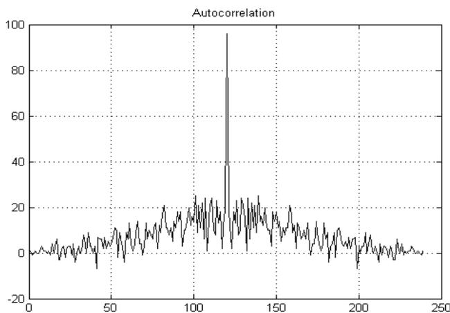
Figure 3: Autocorrelation Function of PN Sequence Generated
