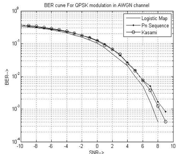
Figure 5: BER curve for QPSK Modulation.
