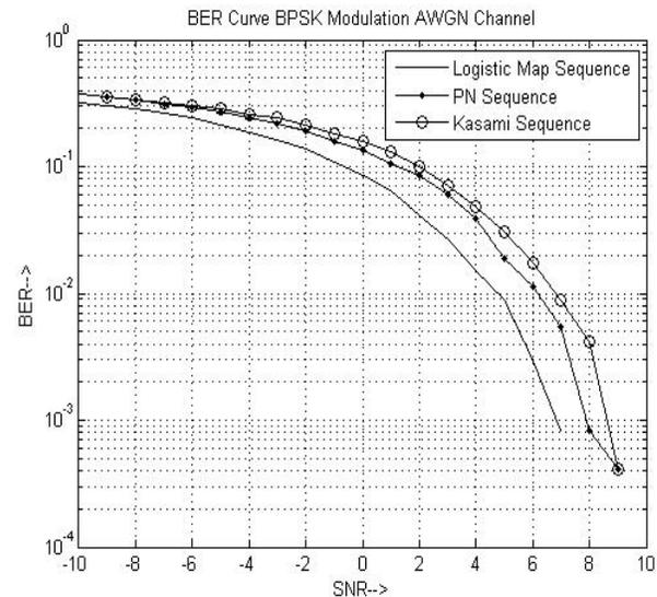
Figure 4: BER curve for BPSK Modulation.
