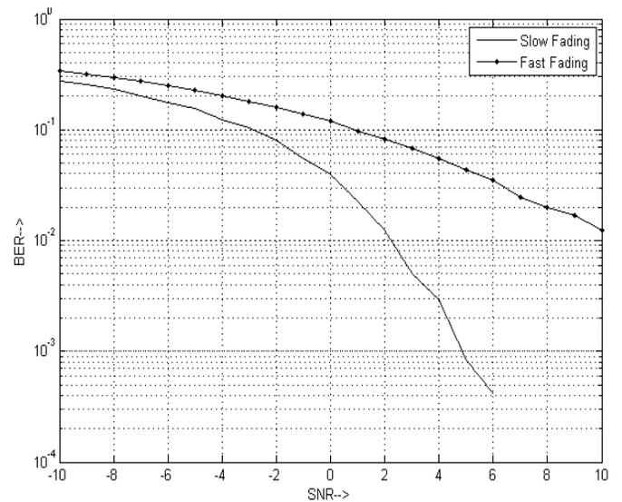
Figure 15: BER curve showing flat fading versus slow fading for QPSK.
