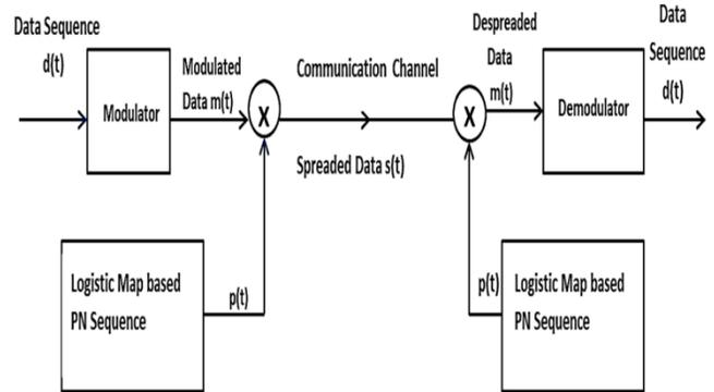
Figure 2: DSSS Modulation Scheme
