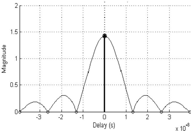
Figure 17: Channel Impulse response for fast fading channel.
