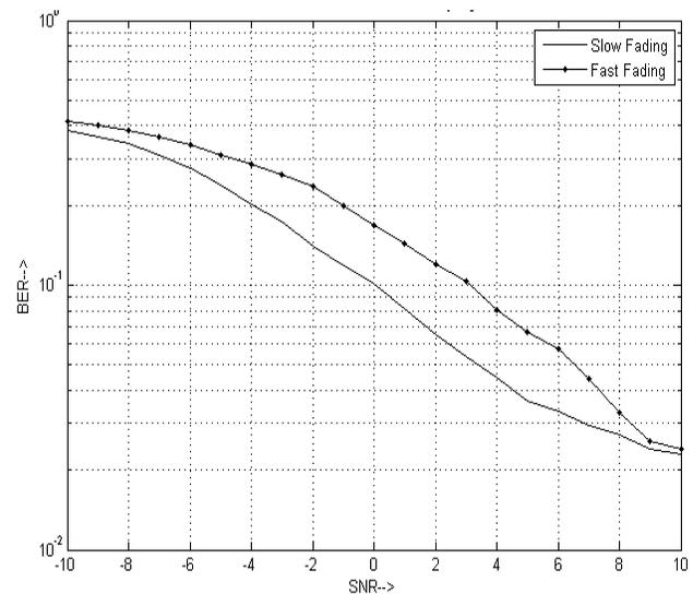
Figure 20: BER curve showing flat fading versus slow fading for DPSK..
