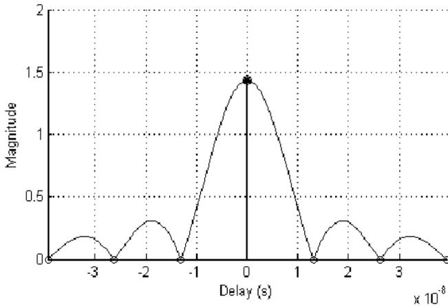
Figure 16: Channel Impulse response for slow fading channel.
