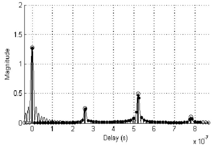
Figure 19: Channel Impulse response for frequency selective fading channel.
