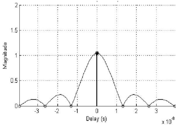
Figure 21: Channel Impulse response for slow fading channel.
