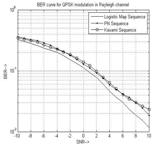
Figure 8: BER curve for QPSK Modulation in Rayleigh Channel.
