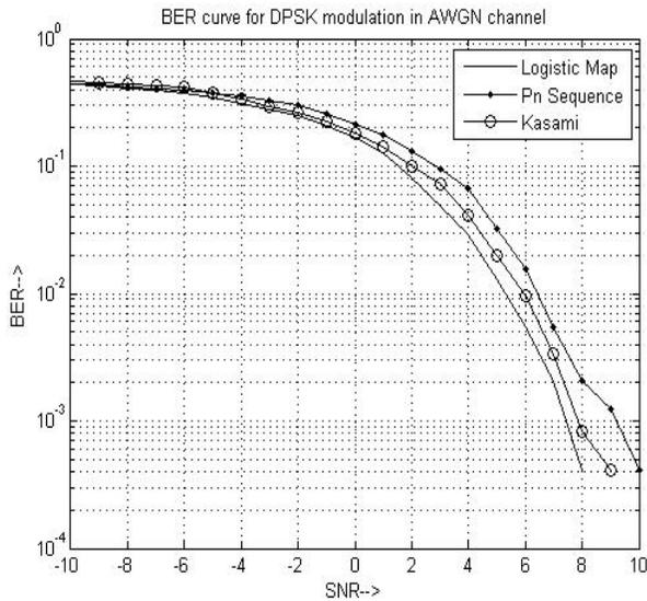
Figure 6: BER curve for DPSK Modulation.
