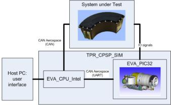
Fig. 3: HIL system scheme
