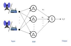
Fig. 1 Architecture of a RBF network in WLAN/GSM system
