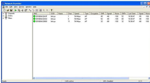
Fig. 3 Network Stumbler application for WLAN data collection
