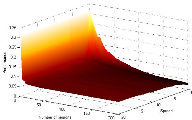
Fig. 7. 3D plot of the training set performance as the function of spread and number of neurons
