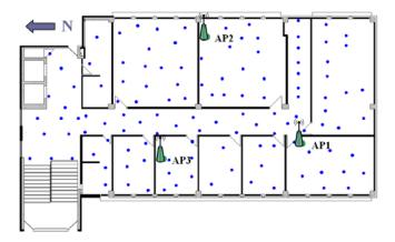
Fig.2 The test location layout with positions of the access points and measurement locations
