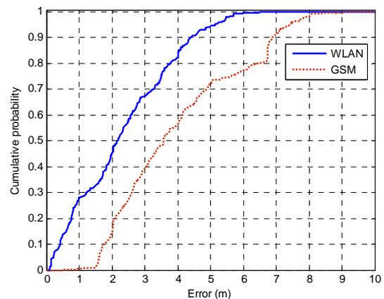
Fig. 11. Cumulative distribution of localization error
