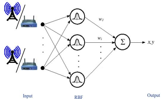
Fig. 1 Architecture of a RBF network in WLAN/GSM system
