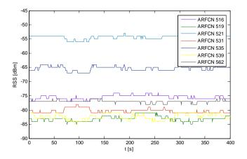
Fig. 6 Measured signal from seven GSM 1800 channels from one GSM provider
