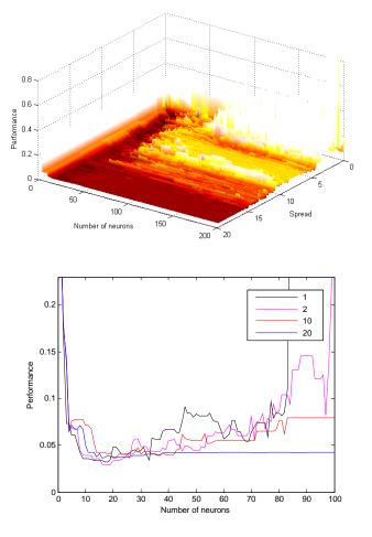
Fig. 8. 3D plot of the validation set performance as the function of spread and number of neurons (top) and validation performance for several single values of spread (bottom)
