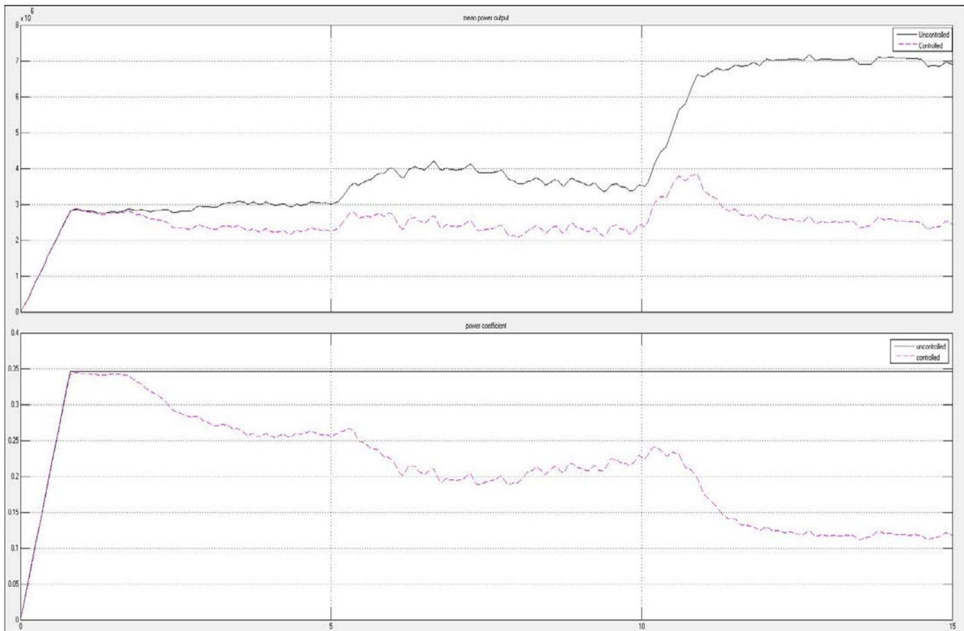
Fig. 9 effect of wind disturbances on output and power coefficient of 2MW turbine under uncontrolled as well as controlled operation with blade pitch angle as five degree
