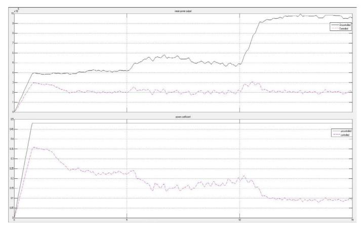
Fig. 8 effect of wind disturbances on output and power coefficient of 2MW turbine under uncontrolled as well as controlled operation with blade pitch angle as zero degree
