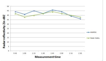
Fig. 5 A Comparison of the Radar Reflectivity Z [dBZ] Parameters of the MMR50 Meteorological Radar and Skalky Meteorological Radar for Convective Precipitation Clouds Formations of June 15, 2013
