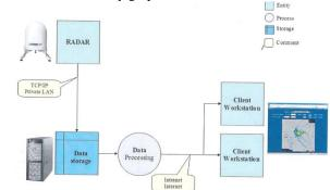
Fig. 1 Scheme of MMR50 Meteorological Radar project [13]
