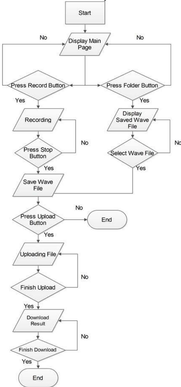
Fig. 6. Overall flowchart of IFSIS Android application
