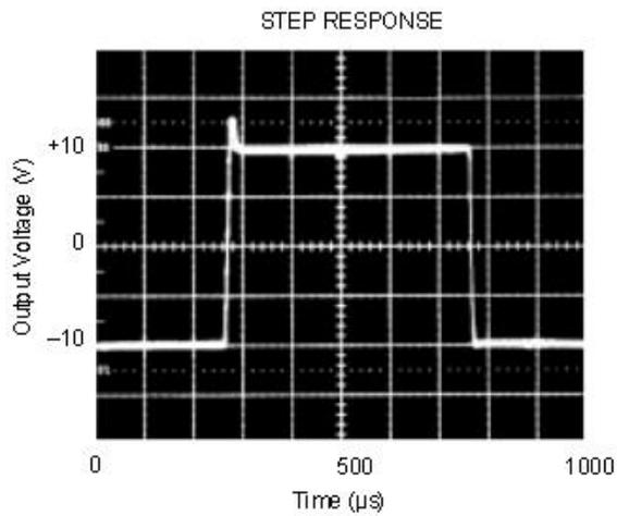
Fig. 6 Step response of ISO124 to a pulse wide  $500 \mu\text{s}$  [3]
