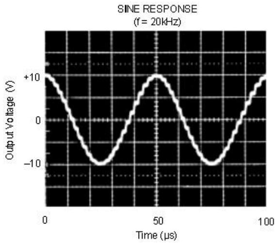
Fig. 5 Sine response of ISO124 on the signal with  $f = 20 \text{ kHz}$  and  $V_{PP} = 20 \text{ V}$  [3]. The effect of sampling can be observed here.
