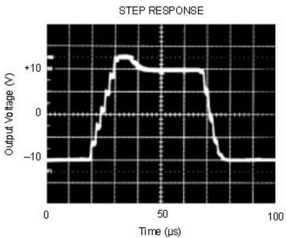
Fig. 7 Step response of ISO124 to a pulse wide  $50 \mu\text{s}$  [3]
