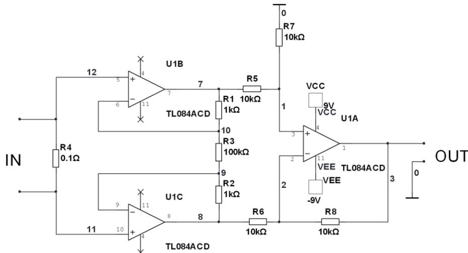
Fig. 21 Suggested instrumentation amplifier – simulation schema
