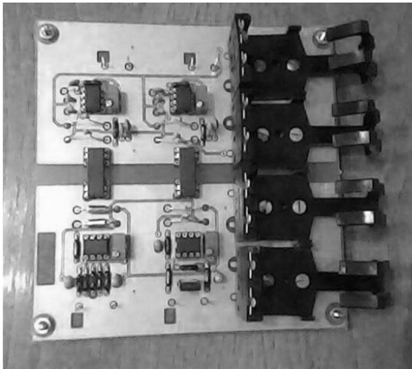
Fig. 12 Battery powered version of the isolating interface
