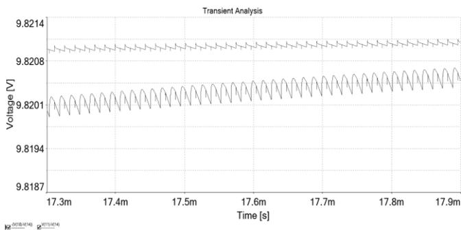
Fig. 18 Voltage ripple at loads of 10 and 20 mA
