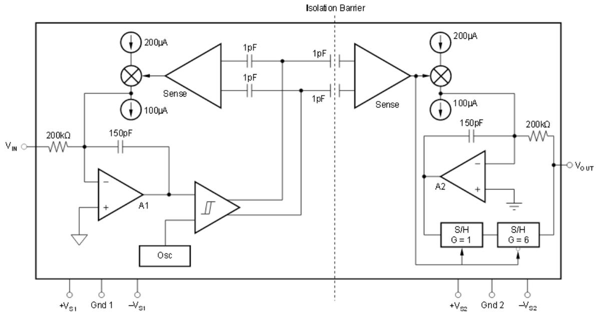
Fig. 2 Block diagram of internal circuits in ISO124 [3]
