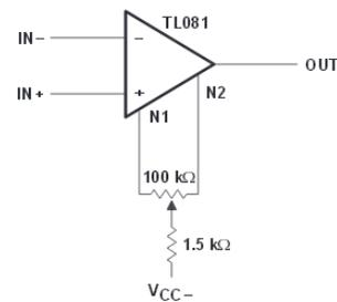
Fig. 8 Basic connection diagram including zero level setting [4]
