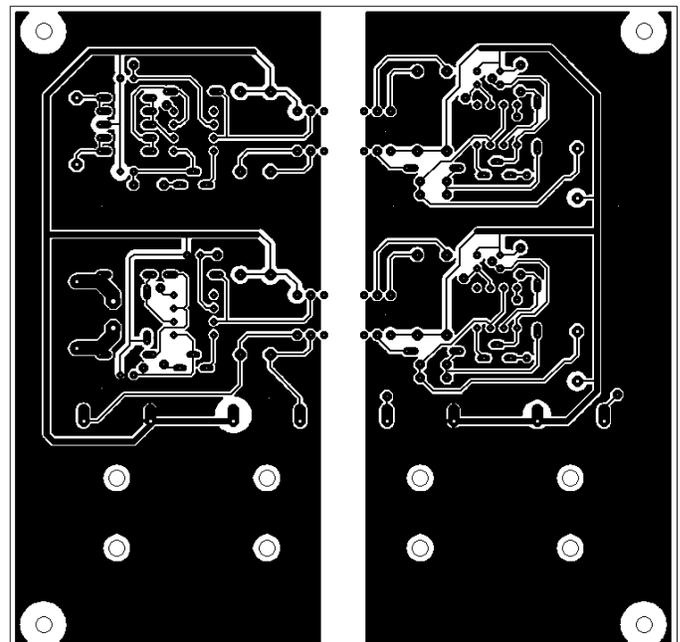
Fig. 14 Printed circuit board – bottom side
