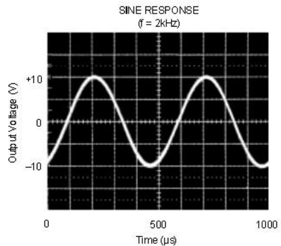
Fig. 4 Sine response of ISO124 on the signal with  $f = 2 \text{ kHz}$  and  $V_{PP} = 20 \text{ V}$  [3]
