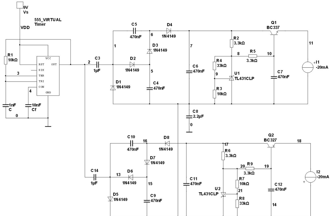
Fig. 16 Symmetrical voltage converter and stabiliser without a DC coupling
