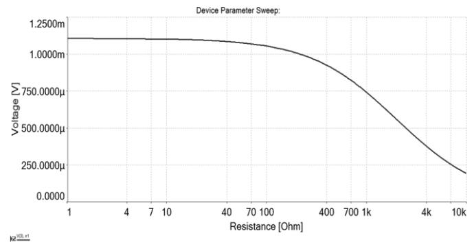
Fig. 20 Dependence of a typical output voltage offset on the value of the resistor R5
