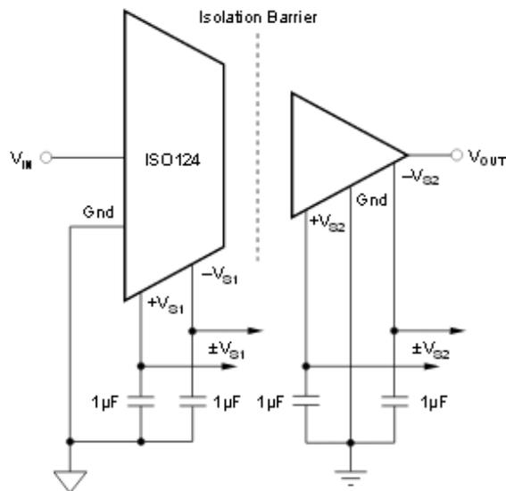
Fig. 3 Basic signal and power connections of ISO124 [3]
