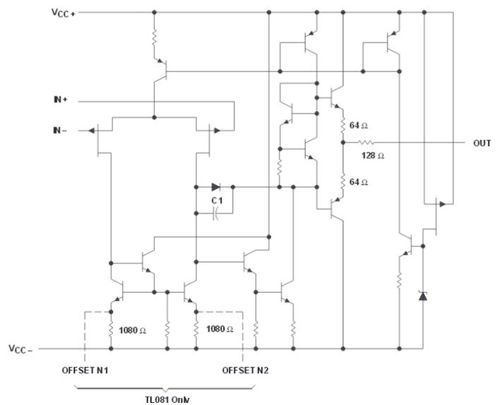
Fig. 9 Internal connection of TL081 [4]
