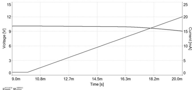
Fig. 17 Output voltage versus load current
