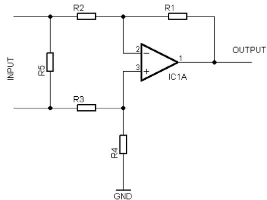
Fig. 19 Connection diagram of a current input of the interface
