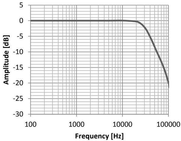
Fig. 11 Typical frequency response of the isolating interface
