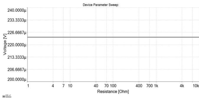
Fig. 22 Dependence of a typical voltage offset of the instrumentation amplifier depicted in Fig 21 on the resistance of the resistor R4
