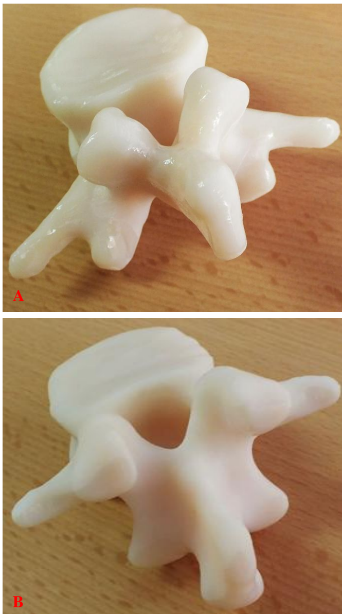
Fig. 16 The final anatomical models with different surface quality. (a) Smooth surface, (b) Matt surface
