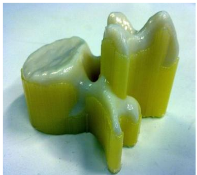
Fig. 15 The 3D models of spinae vertebrae with the support material
