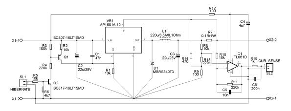
Fig. 11 Connection diagram of Step-down converter with AP1501A-12
