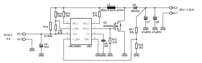
Fig. 15 Connection diagram of Step-up converter with MC34063
