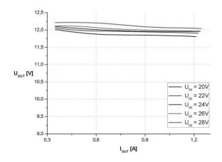
Fig. 16 Output voltage of the converter vs. output current
