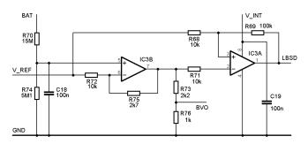
Fig. 10 Connection diagram of the Battery monitor
