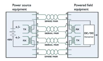
Fig. 1 Power over Ethernet principle [7]
