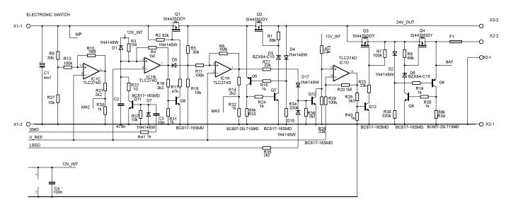
Fig. 6 Connection diagram of the Electronic switch
