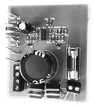
Fig. 20 Electronic switch functional sample
