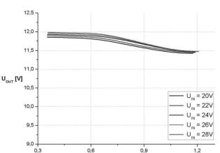
Fig. 12 Output voltage of the converter vs. output current
