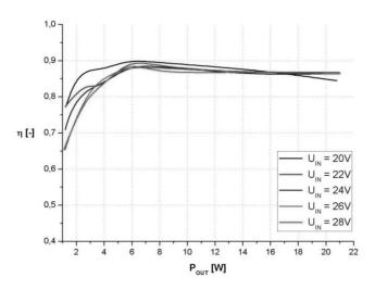
Fig. 19 Power efficiency of the converter vs. output power
