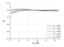
Fig. 17 Power efficiency of the converter vs. output power
