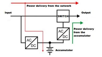
Fig. 3 Off-line UPS block diagram [2]
