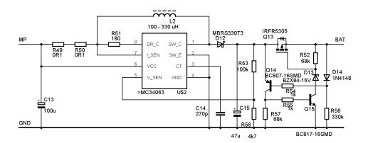
Fig. 8 Connection diagram of Battery charger
