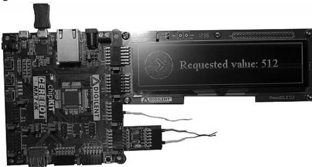
Fig. 13 The Cerebot hardware with connected peripheral modules
