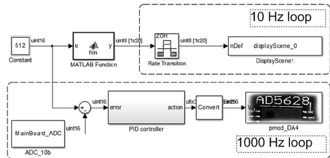
Fig. 14 Simulink scheme of algorithm implemented in Cerebot
