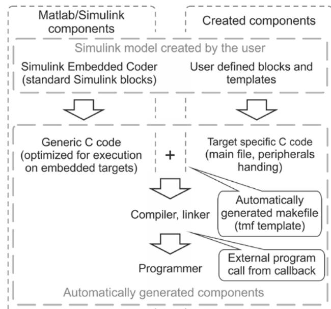
Fig. 5 Simulink model and components for code generation
