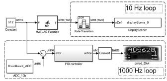
Fig. 14 Simulink scheme of algorithm implemented in Cerebot
