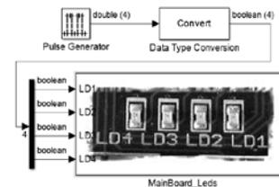
Fig. 7 Identifying block inputs and corresponding led location on board is simple
