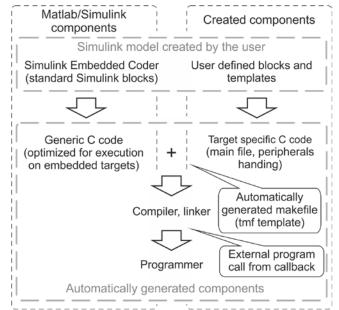
Fig. 5 Simulink model and components for code generation
