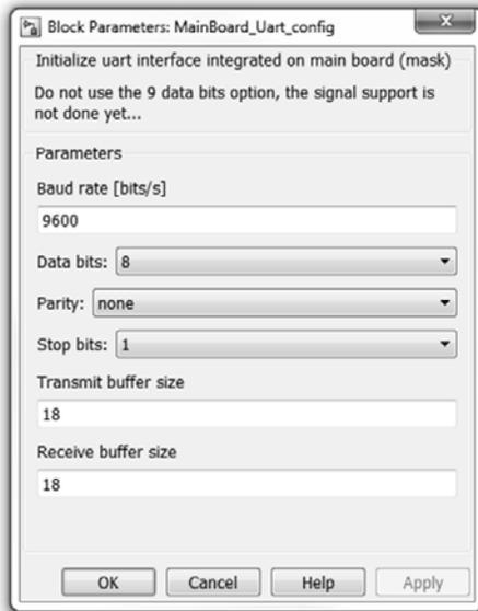
Fig. 9 Dialog for configuring UART peripheral module
