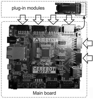
Fig. 2 Cerebot main board with plug in module
