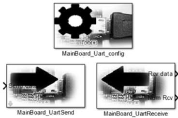
Fig. 8 Blocks and user interface for UART peripheral
