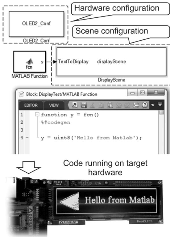
Fig. 10 Code generated from Simulink running on target hardware
