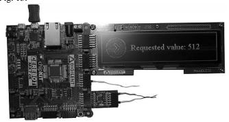
Fig. 13 The Cerebot hardware with connected peripheral modules
