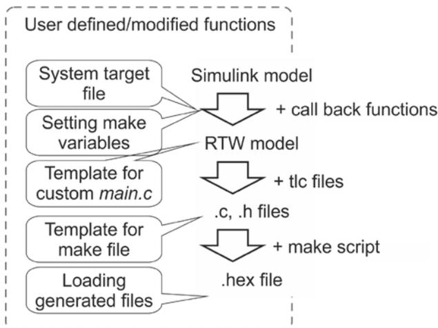
Fig. 4 User defined files used during various stages of code generation process
