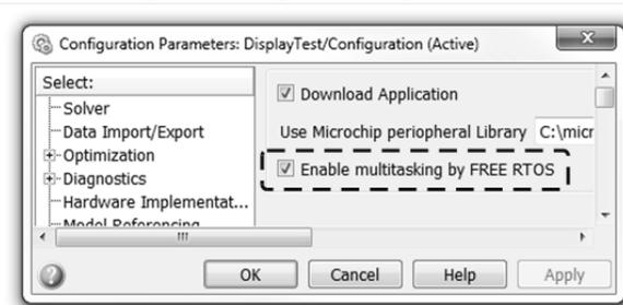
Fig. 6 Enabling option for generating preemptive code powered by a Free RTOS from Simulink model
