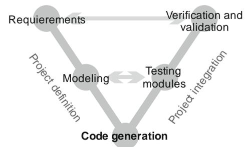
Fig. 1 Automatic code generation in context of development cycle
