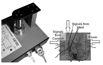
Fig. 12 Overview controlled plant (left) and signal conditioning circuits (right)
