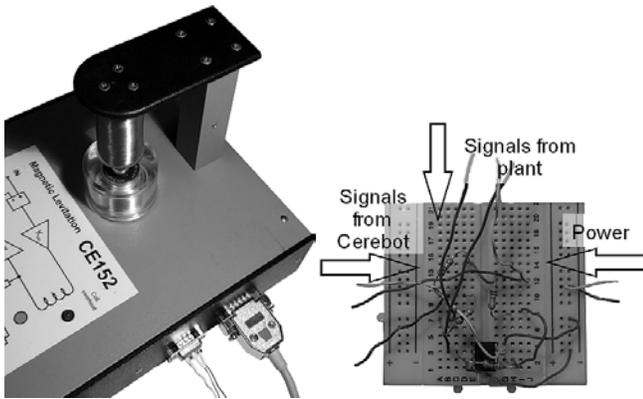
Fig. 12 Overview controlled plant (left) and signal conditioning circuits (right)
