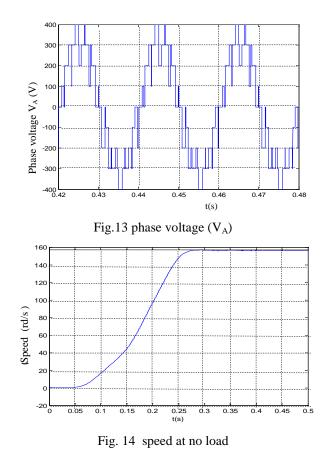
V. EXPERIMENTAL TESTS OF THE NPC INVERTER
