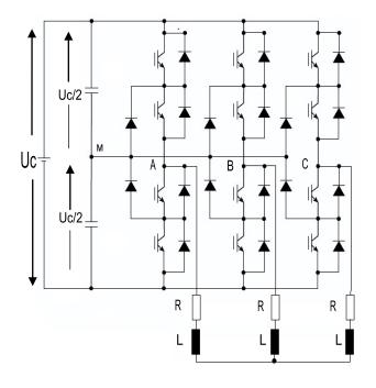
Fig.1. Power circuit of NPC inverter
