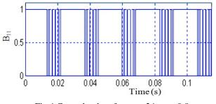
Fig.4 Control pulses for  $m_f=24$   $m_a=0.8$
