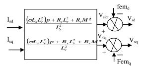
Fig.11 Decoupling control
