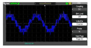
Fig.17 Output voltage of phase VA(15V/Div)
