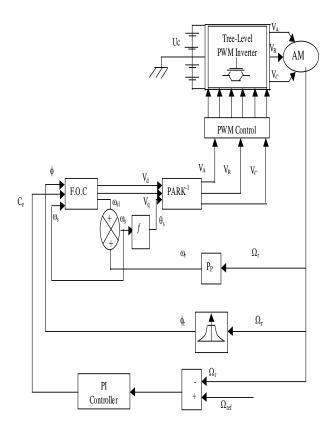
Fig.12 Block diagram of the indirect field oriented induction motor drive system fed by three – level PWM inverter with PI controller.
