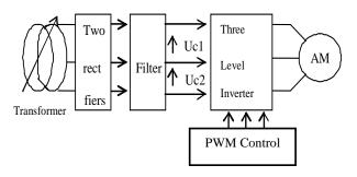
Fig.20 Block diagram A.M fed PWM
