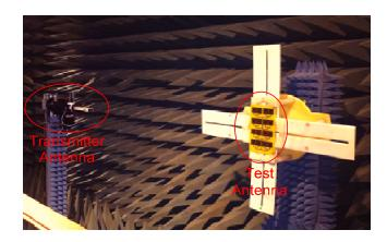
Fig. 7. Test antenna installed at test gauge in anechoic chamber room.
