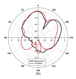
Fig. 11. Proposed antenna radiation patterns (a) E-field (b) H-field.
