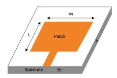
Fig. 1. Basic microstrip antenna.
