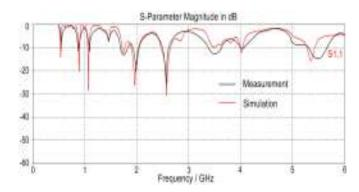
Fig. 9. Proposed array antenna reflection coefficient.
