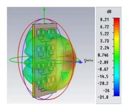
Fig. 10. Array LTE antenna radiation pattern in 3D.
