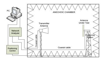
Fig. 6. Block diagram of measurement setup.
