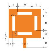
Fig. 2. Single patch antenna design with slots.
