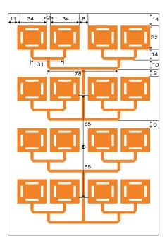
Fig. 3. Proposed high gain array antenna. (NB: All dimensions are in mm)
