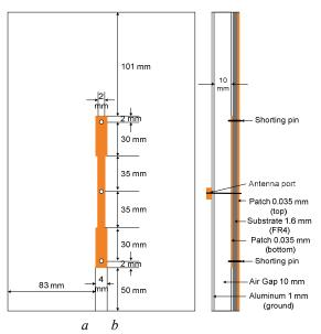
Fig. 4. Proposed antenna structure (a) FR4 back view (b) Side view.
