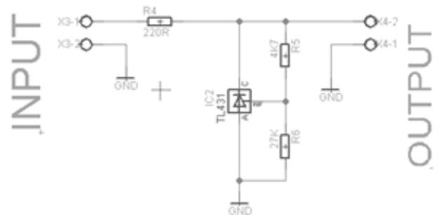
Fig. 6 Circuit with the voltage reference TL431
