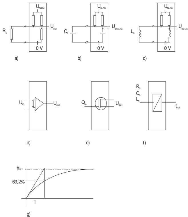
Fig.5 Scheme of converting the primary sensor signal into voltage
