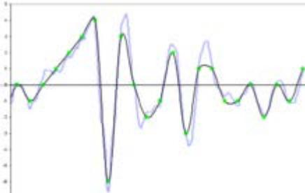
Fig 13 Reconstruction of analog signal from digital data.
