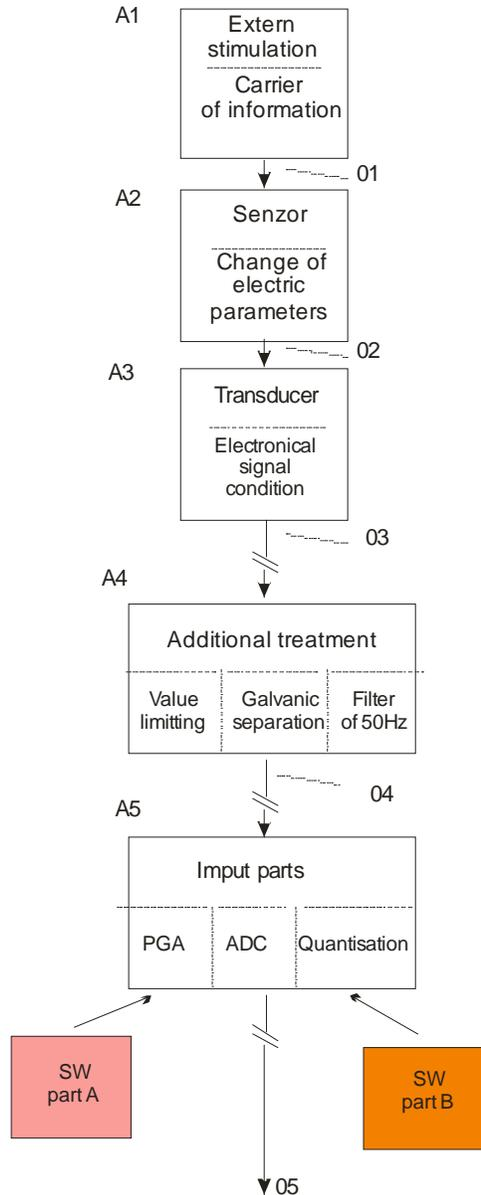
Fig. 3 Scheme of input part of signal condition
