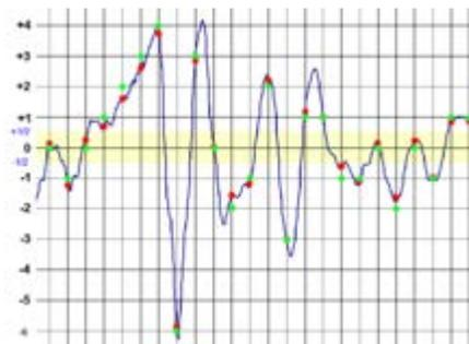
Fig.12 Scheme of quantification of signal samples
