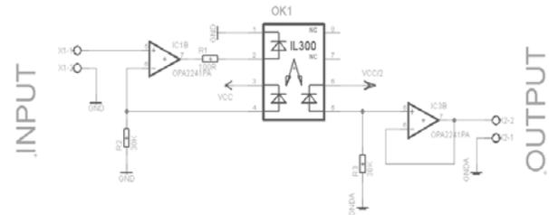
Fig.9 Circuit with the optocoupler IL300
