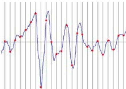
Fig. 11 Scheme of sampling of analog signal of speech sound „A”
