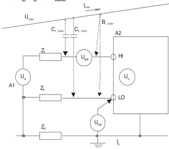
Fig.8 Influence of interference voltage to measured signal
