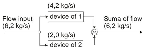
Fig.14 Pipe system with balanced flow date.
