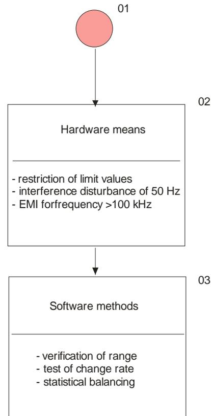
Fig. 2 Block scheme of signal condition of sensors
