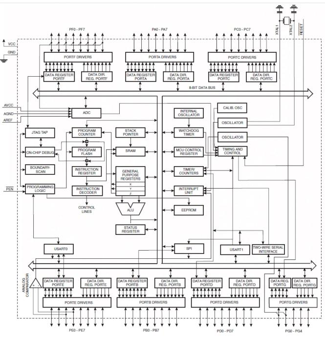
Fig. 1 Block Diagram of the AVR Architecture [5]
