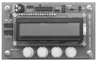
Fig. 4 LCD module with control buttons [17]
