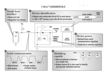
Fig. 10 1-Wire Bus basic circuit [19]
