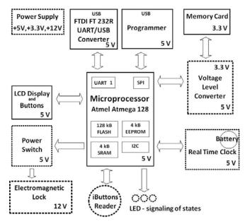
Fig. 7 Block Diagram of the Access System
