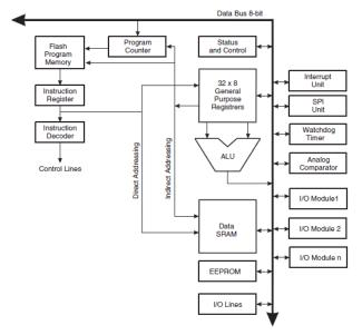
7Fig. 2 Block Diagram of the AVR Architecture [5]
