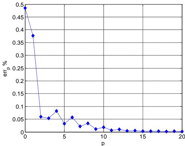
Fig. 8 First stroke lightning base current in the frequency domain: error as function of the number of coefficients.
