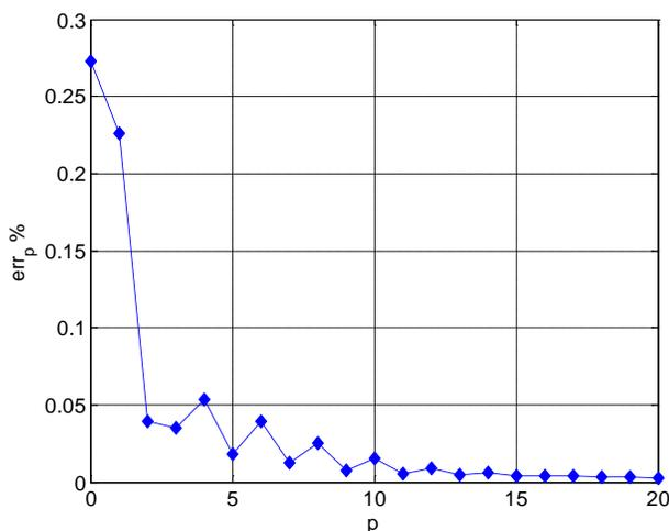
Fig. 9 Subsequent stroke lightning base current in the frequency domain: error as function of the number of coefficients.
