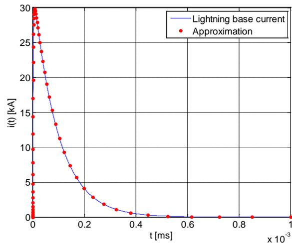
Fig. 2 First stroke lightning base current in time domain: comparison between analytical expression (4) and approximation ( $p = 0-10$ ).
