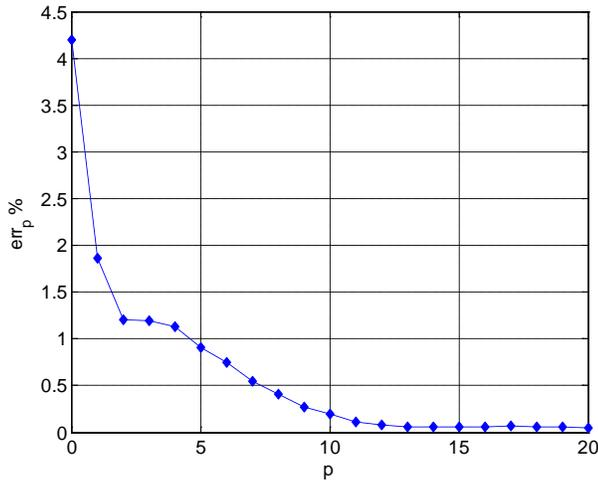
Fig. 4 First stroke lightning base current in time domain: error as function of the number of coefficients.
