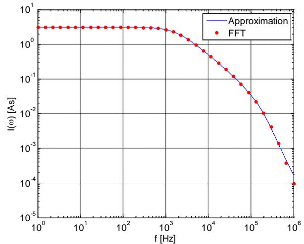
Fig. 6 First stroke lightning base current in the frequency domain: comparison between FFT and approximation ( $p = 0-10$ ).
