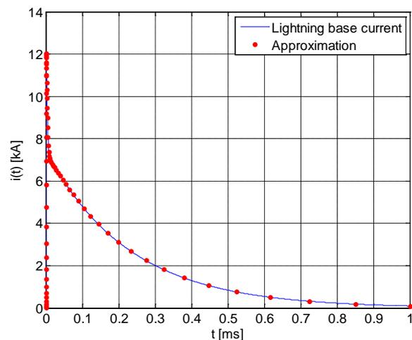
Fig. 3 Subsequent stroke lightning base current in time domain: comparison between analytical expression (4) and approximation ( $p = 0-10$ ).
