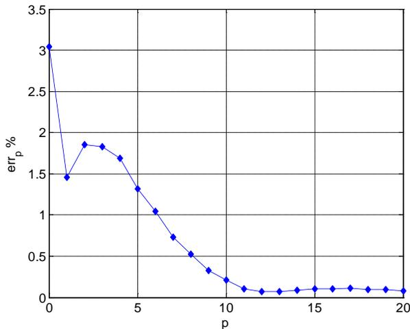
Fig. 5 Subsequent stroke lightning base current in time domain: error as function of the number of coefficients.
