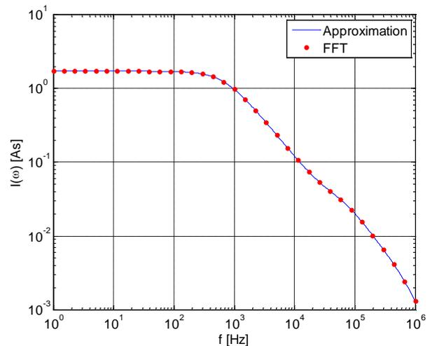
Fig. 7 Subsequent stroke lightning base current in the frequency domain: comparison between FFT and approximation ( $p = 0-10$ ).
