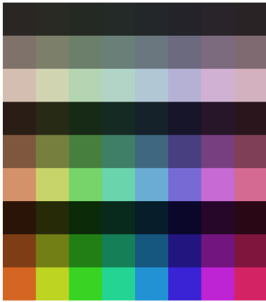
Fig. 1: The significant colors of bins based on the HSV color space. The H channel is divided into 8, the S and V channel into 3-3 equally wide intervals.
