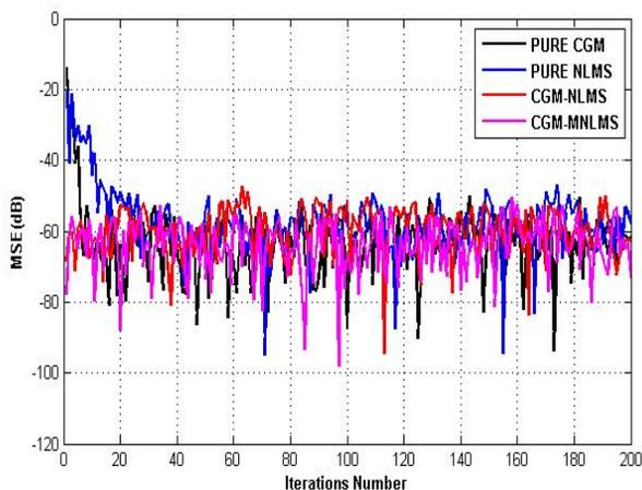
Fig. 9 MSE plot for all algorithms / Rayleigh channel
