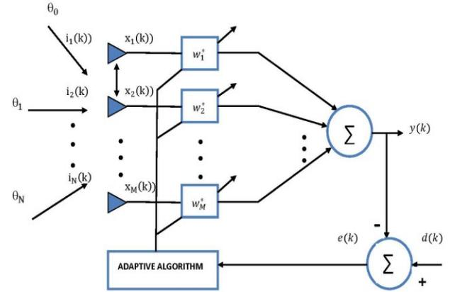
Fig. 1. Block diagram of Smart Antennas System.
