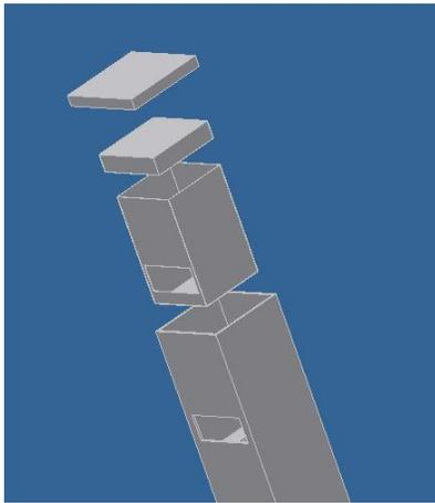
Fig. 7 Modelled rack with folding shielding box for camera
