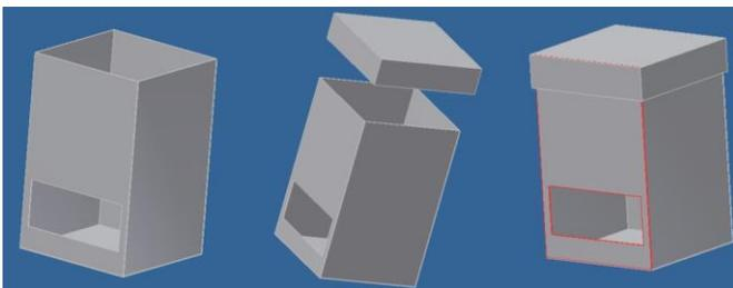
Fig. 4 Sample of modeled shielding box with a lid
