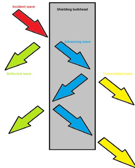
Fig. 1 Multiple reflections at the input and output shielding bulkhead [5]
