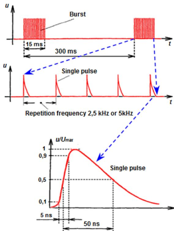
Fig. 2 The course of electrical fast transients [1]
