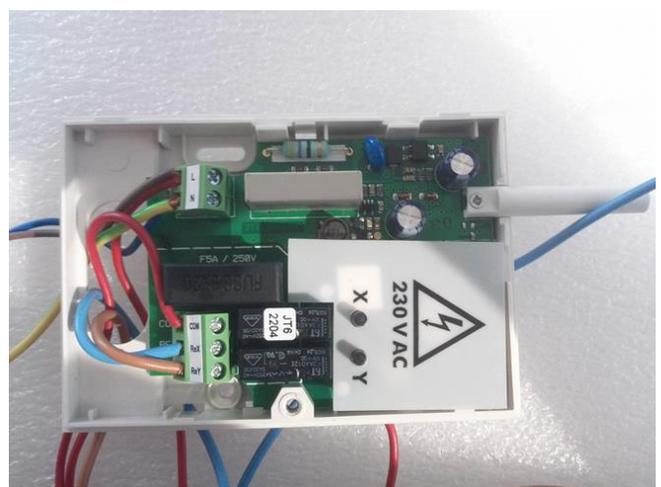
Fig. 6 Wireless relay AC82
