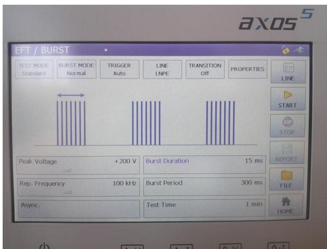
Fig. 7 AXOS 5 - setting of testing EFT/B
