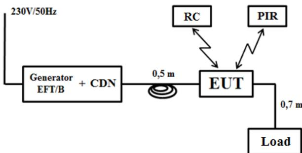
Fig. 4 Diagram of the proposed workplace for the testing EMS
