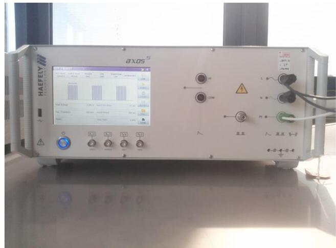
Fig. 5 Testing device AXOS5
