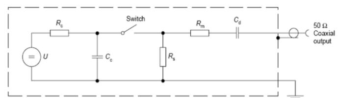
Fig. 3 Simplified diagram of the generator of the electrical fast transient/burst
