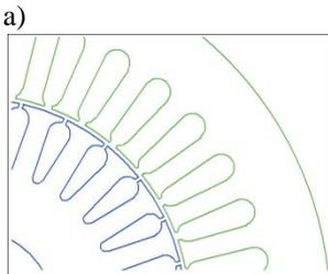
Fig. 1 a) general view and b)stator and Rotor slot shapes of the designed IM
