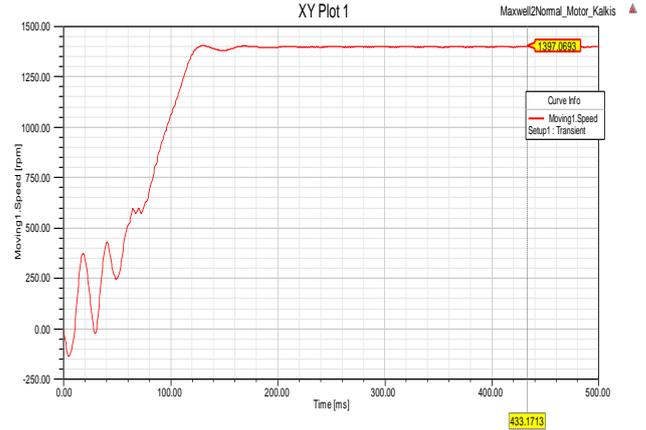
c) Fig. 8 (continued) transient variations for balanced stator voltages c) shaft speed
