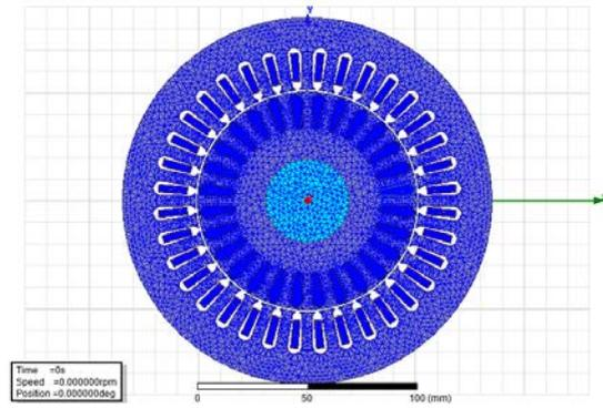
Fig. 6 finite elements mesh for the transient analysis
