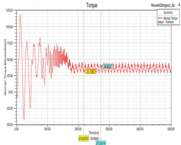
a) Fig. 9 Transient variations for unbalanced stator voltages. a)Electromagnetic torque
