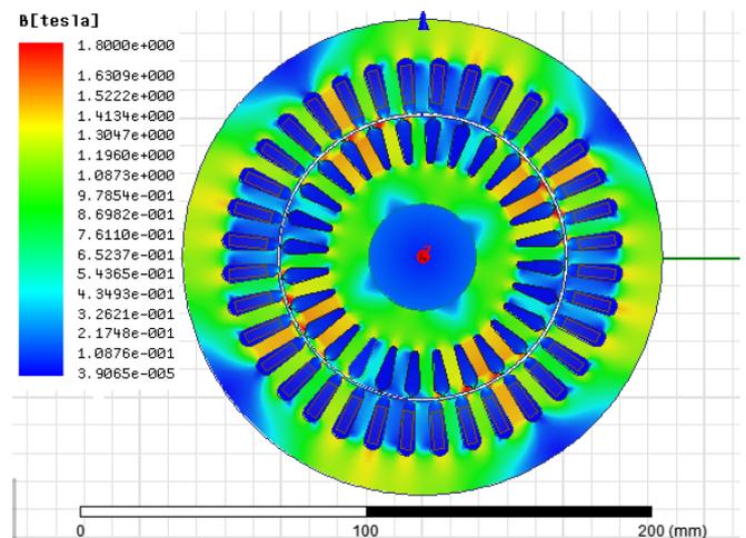
Fig.7. Instantaneous field distribution over the stator and rotor
