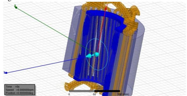
Fig. 12 Rotor bar skew and its angular direction
