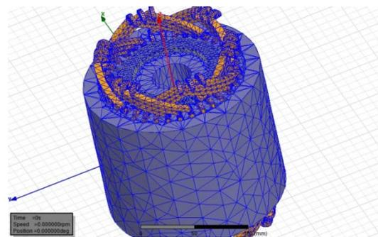
Fig. 11 3D Mesh of the induction motor
