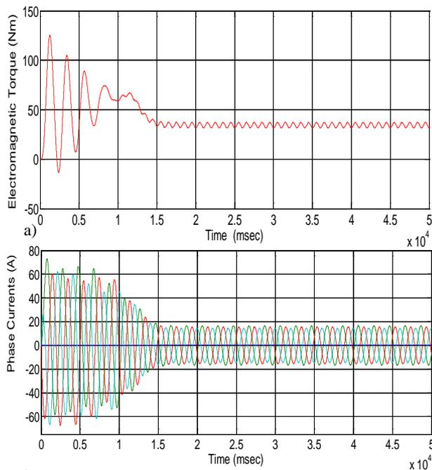
Fig. 10 Transient variations for unbalanced stator voltages which are obtained by solving d,q,0 model a) electromagnetic torque, b) stator current
