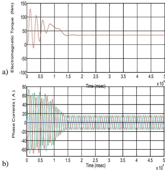
Fig. 4 solution of d,q,0 model for balanced voltage and rated loaded starting a)electromagnetic torque b) phase currents
