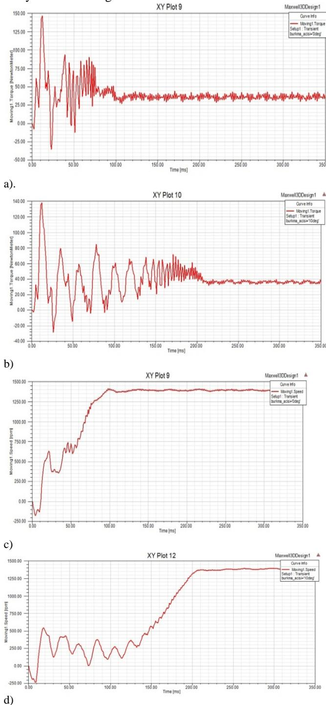
Fig. 13 3D transient FEA results for two rotor bar skew
